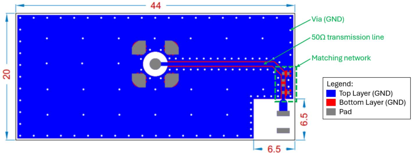
Detailed view of antenna pads and copper clearance:
