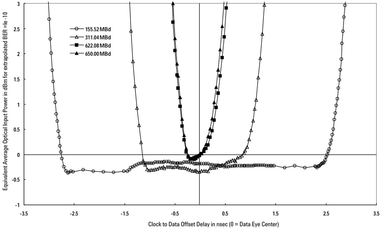
Figure 2. HFBR-5208xxMZ Relative Input Optical Power as a function of sampling time position. Normalized to center of Baud interval at 622 MBd. Test Conditions +25°C, 5.25 V, PRBS 2<sup>23</sup>-1, optical  $\tau_r/\tau_f = 0.9$  ns with 3 m of 62.5  $\mu$ m MMF.
