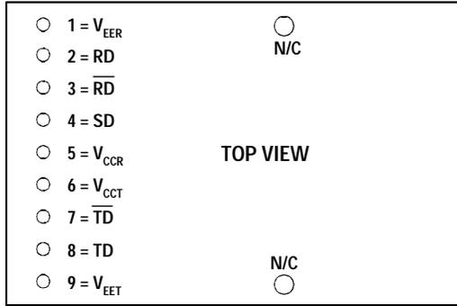
N/C = NO INTERNAL CONNECTION (MOUNTING POSTS) - CONNECT TO CHASSIS GROUND OR LEAVE FLOATING, DO NOT CONNECT TO SIGNAL GROUND.
