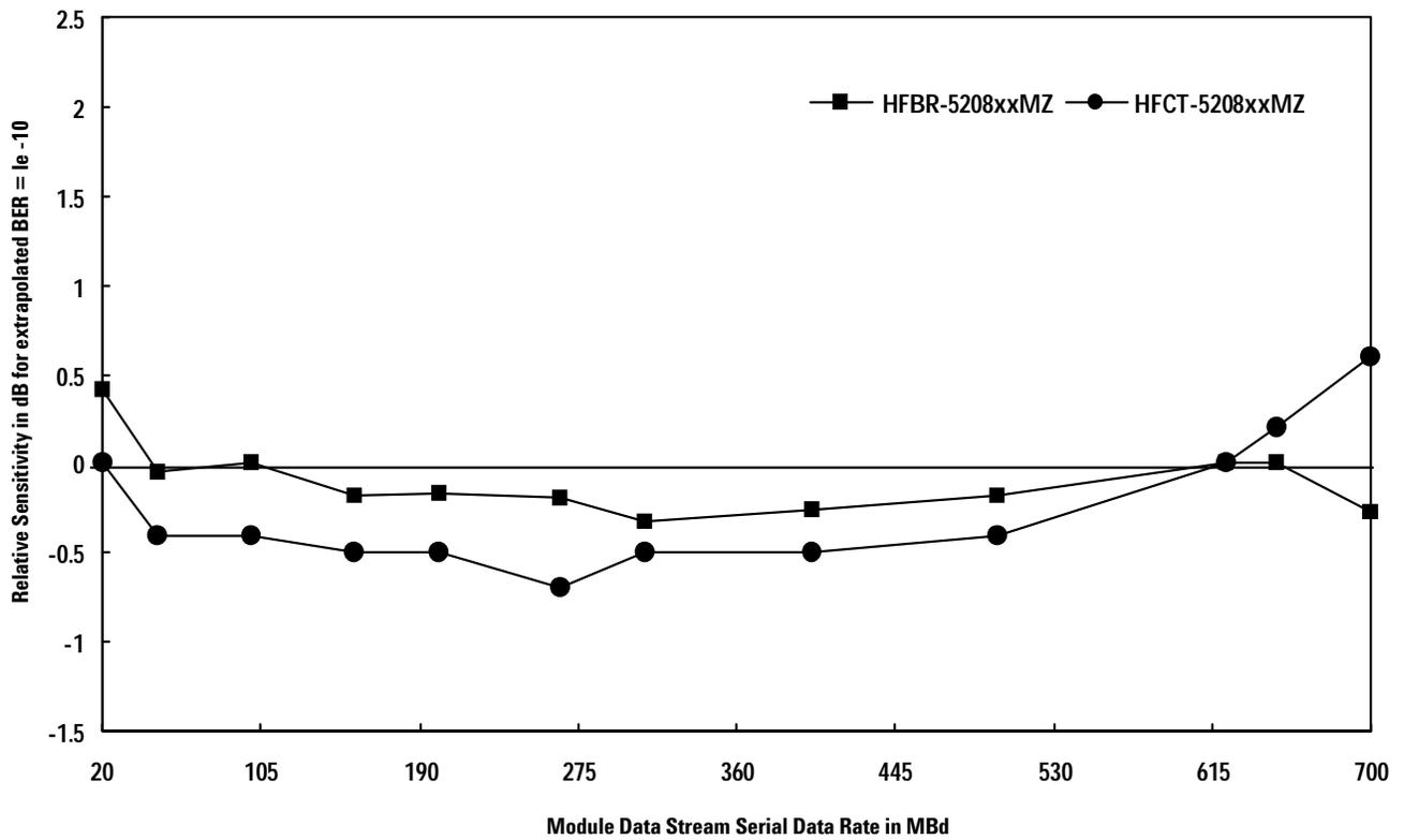
Figure 3. Relative Input Optical Power as a function of data rate normalized to center of Baud interval at 622 MBd. Test Conditions +25°C, 5.25 V, PRBS 2<sup>23</sup>-1, optical  $\tau_r/\tau_f = 0.9$  ns with 3 m of MMF or SMF.
