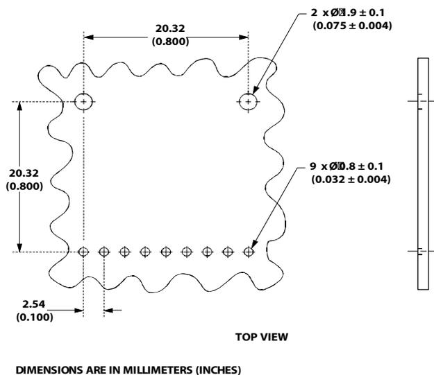
Figure 5. Recommended Board Layout Pattern
