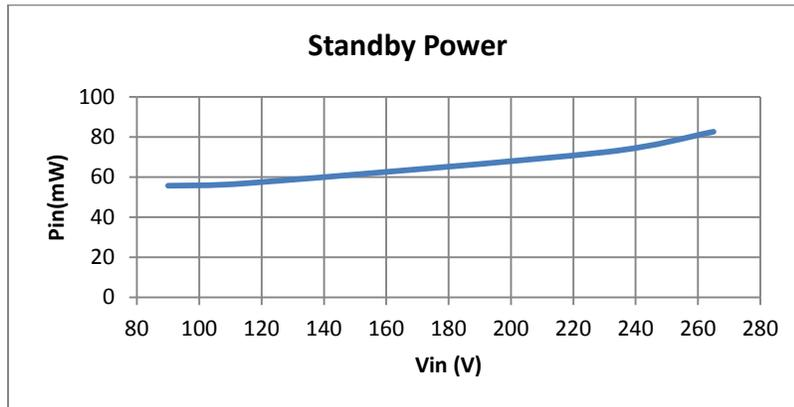
Fig. 7, Standby Power versus Vin Curve
