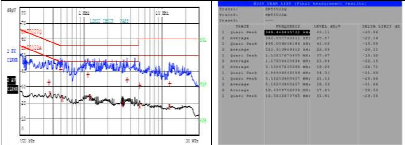
Fig. 41, L line conduction waveform@230V, full load.
