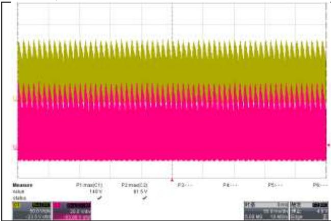
Fig. 19, MOS drain-source 140V, Vak 61V@85V/60Hz, full load
