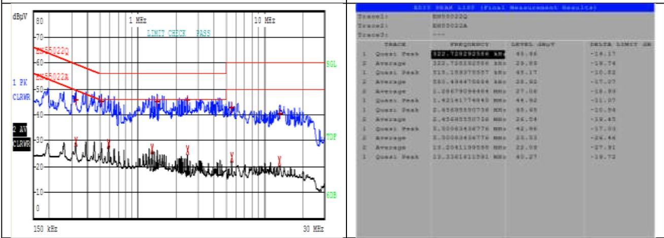
Fig. 43, N line conduction waveform@230V, full load.
