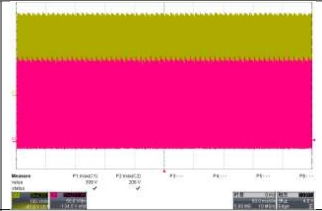
Fig. 22, MOS drain-source 399V, Vak 206V@264V/50Hz, full load
