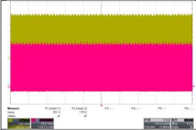
Fig. 21, MOS drain-source 351V, Vak 179V@230V/50Hz, full load
