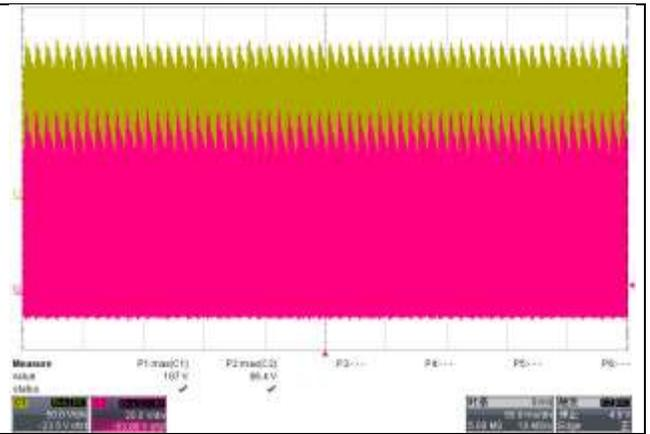
Fig. 20, MOS drain-source 187V, Vak 86V@115V/60Hz, full load
