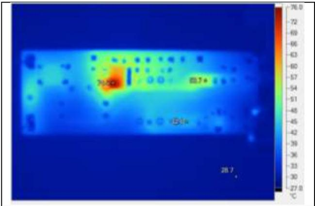
Fig. 39, IC 74.5°C, free-wheeling diode 53.7°C, flyback diode 42.5°C @full load, 85V/60Hz, ambient temperature 28.7°C.
