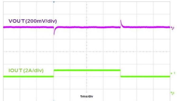
**Figure 8. Output Voltage Ripple, IOUT=3.5A**
