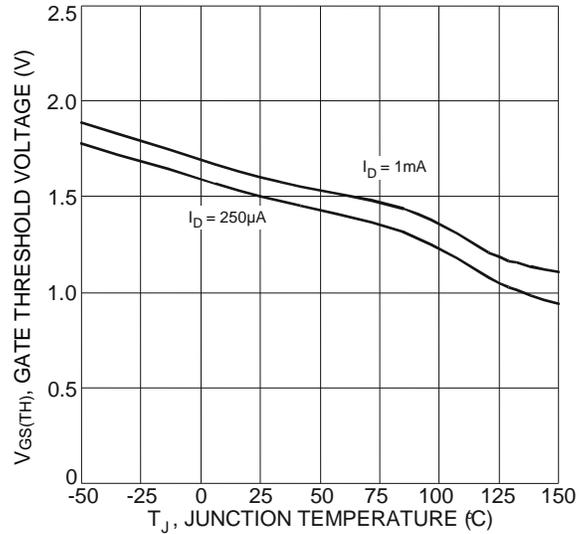
Fig. 11 Gate Threshold Variation vs. Junction Temperature
