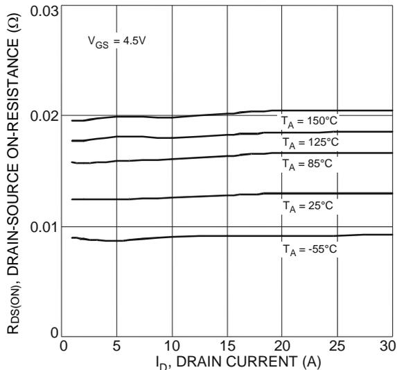
Fig. 8 Typical On-Resistance vs. Drain Current and Temperature
