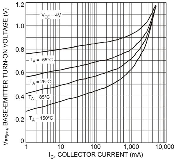
Figure 3 Typical Base-Emitter Turn-On Voltage vs. Collector Current
