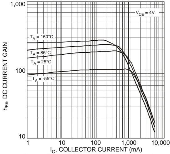
Figure 1 Typical DC Current Gain vs. Collector Current
