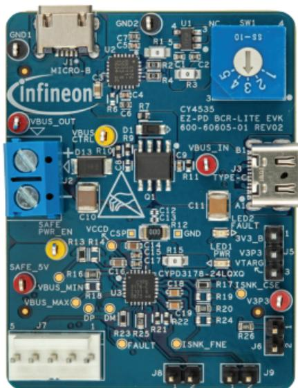
The CY4535 EZ-PD™ barrel connector replacement-lite (BCR-LITE) EVK is an evaluation platform for customers who want to replace an existing barrel/power input connector with a USB-C connector using the CYPD3178 device. Implementing this solution in an end-product allows the system to be powered by any USB Type-C compliant power adapter or USB power adapter that supports legacy charging standards.
