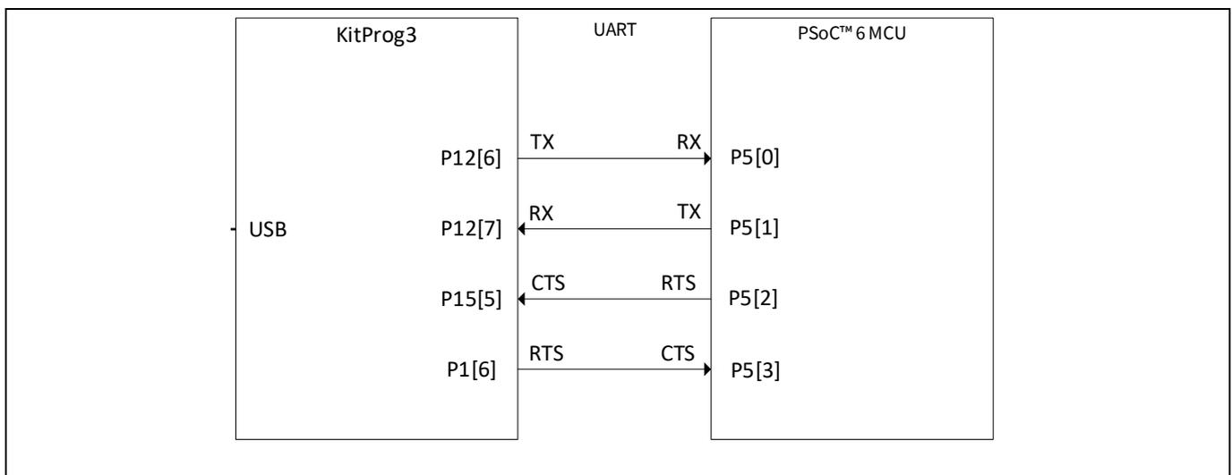
**Figure 9** UART connection between KitProg3 and PSoC™ 6 MCU
