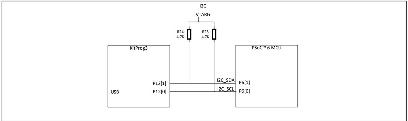
**Figure 10** I2C connection between KitProg3 and PSoC™ 6 MCU
