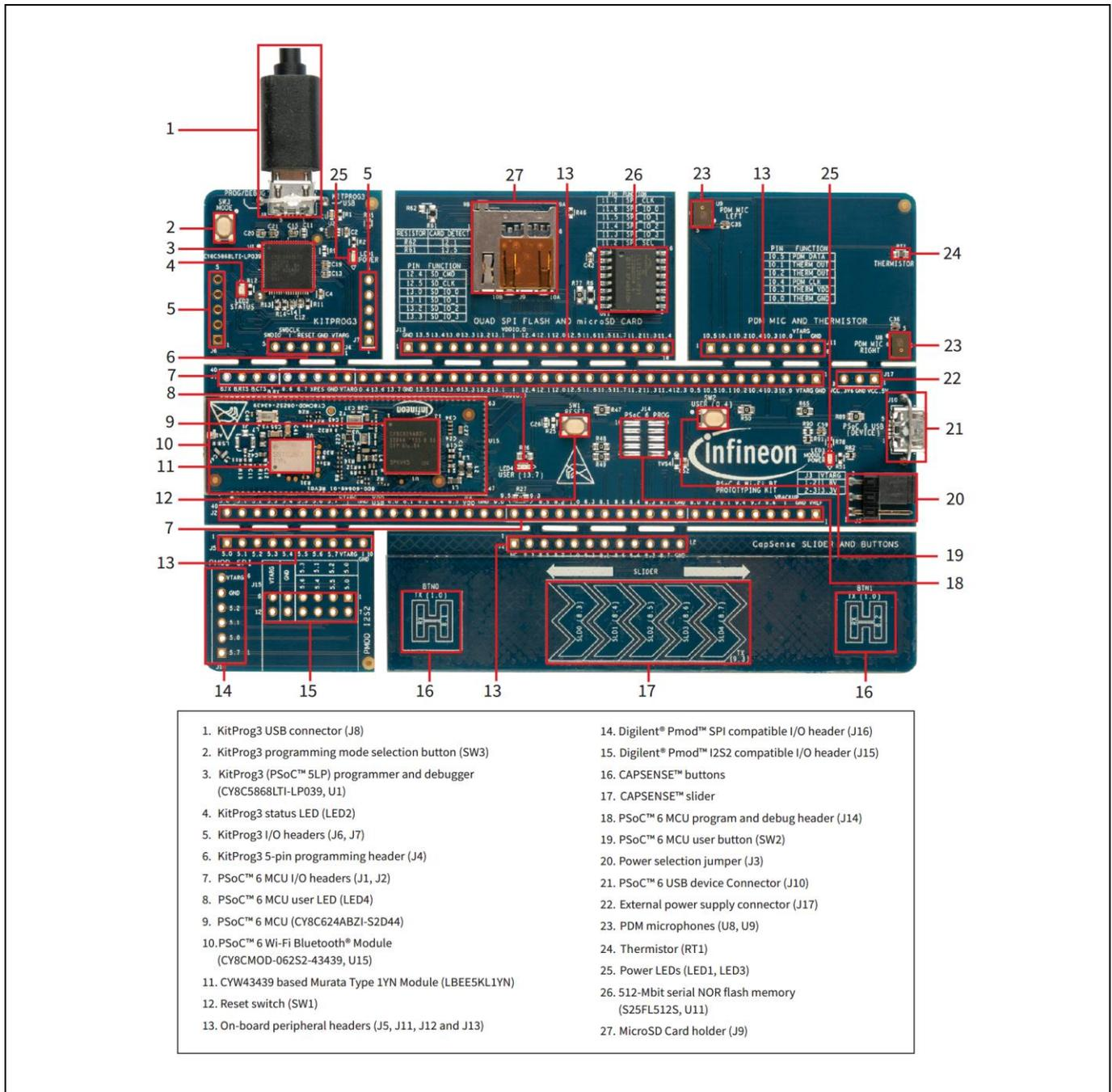
**Figure 1 Board components**
