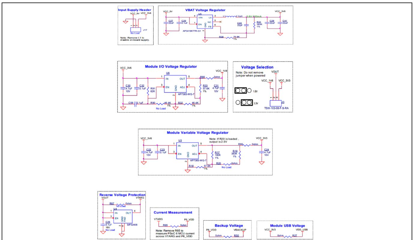
**Figure 14** Schematics of power supply system
