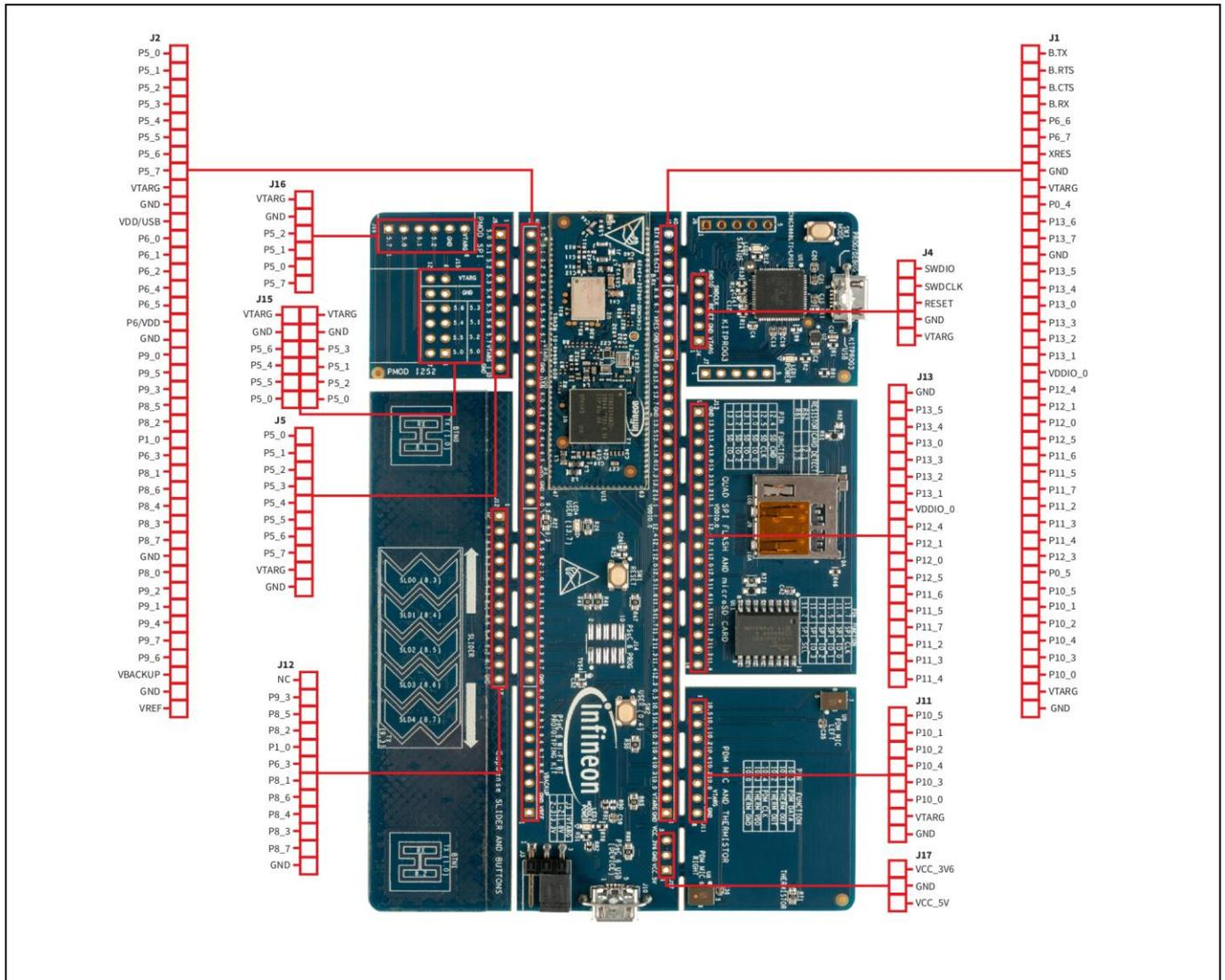
**Figure 2** Prototyping board pinout
