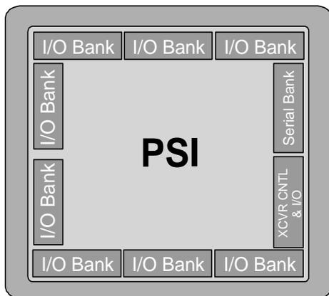
**Figure 9. PSI I/O Bank Block Diagram**
