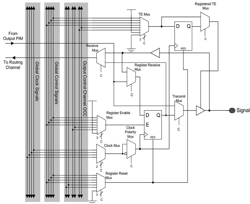
**Figure 3. Block Diagram of a Standard Datapath Cell**
