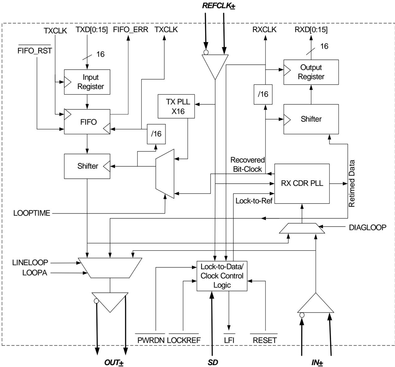
**Figure 13. High-speed PSI Transceiver Logic Block Diagram<sup>[2]</sup>**
