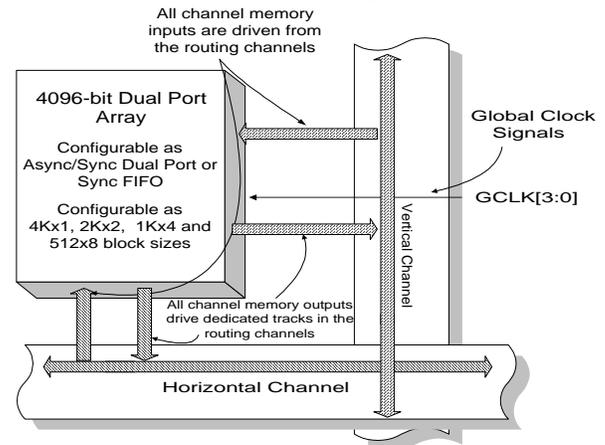
**Figure 8. Block Diagram of Channel Memory Block**
