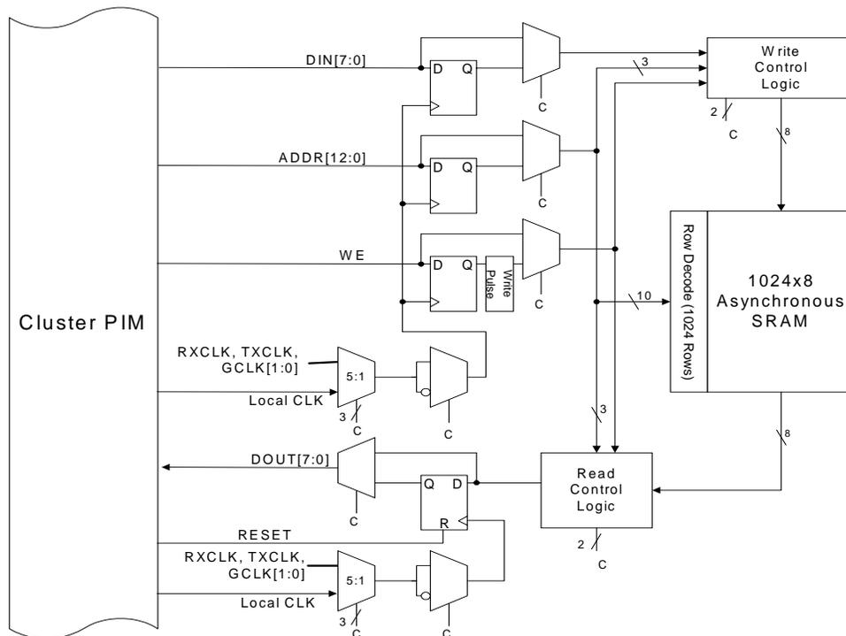
**Figure 7. Block Diagram of Cluster Memory Block**
