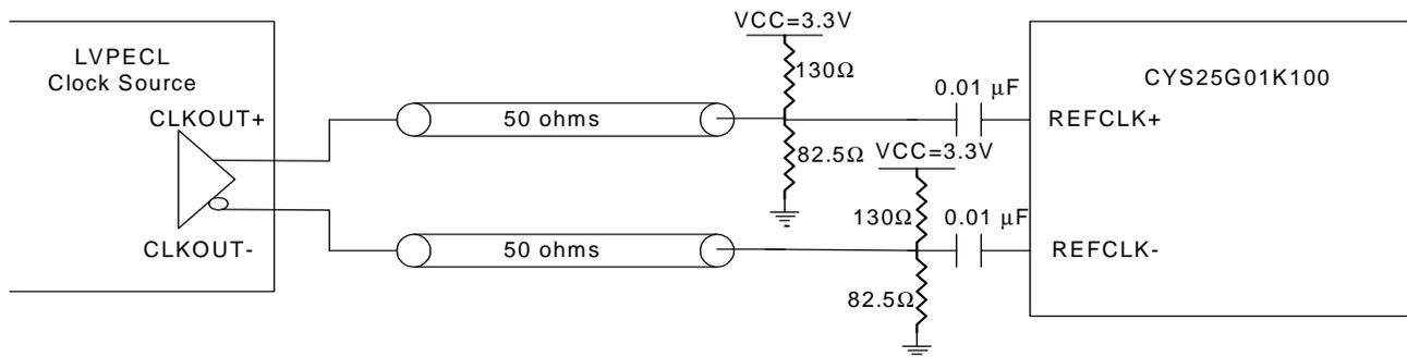
**Figure 22. AC-Coupled REFCLK Oscillator Termination**
