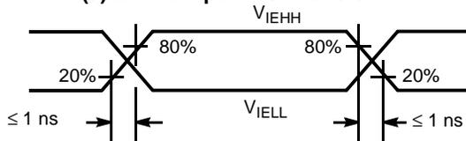
(c) LVPECL Input Test Waveform
