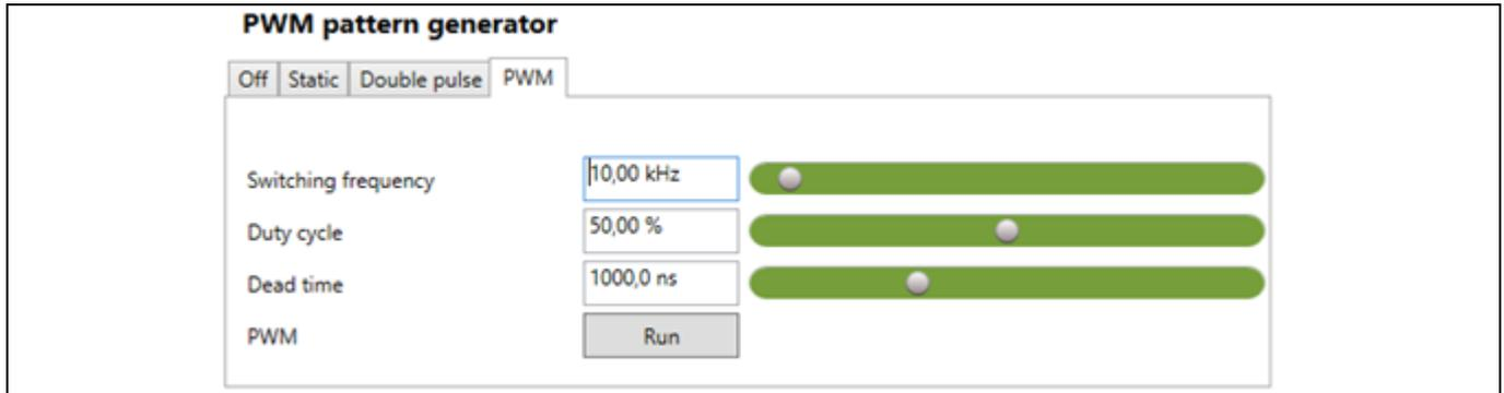
**Figure 35** PWM mode of PWM pattern generator
