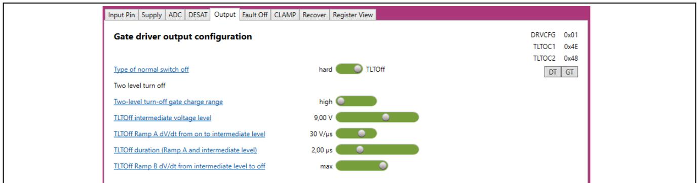
**Figure 19** Output settings of the gate driver
