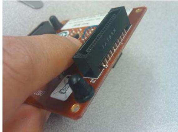
4. Bend the tip of the wire and hook it to the outmost top pin in the P2 connector as shown in the picture.
