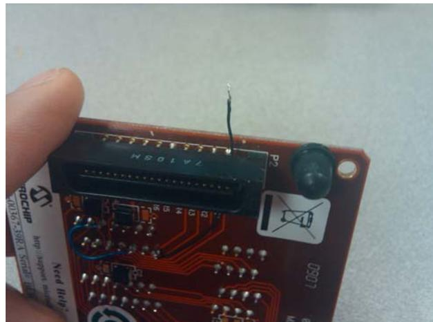
3. Now, run the wire thru the top of the P2 connector as shown in the picture.
