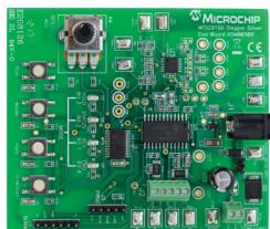
The MTS2916A Dual Full-Bridge Stepper Motor Driver Evaluation Board demonstrates the capabilities of the MTS2916A to control both windings of a bipolar stepper motor. The board also demonstrates the capabilities of controlling two brushed DC motors.
