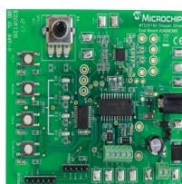
This evaluation board includes push-button switches and a variable-speed input potentiometer to demonstrate the MTS2916A controlling a stepper motor in full-step, half-step, modified half-step and micro-stepping modes.
