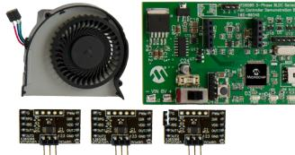
This board allows for the control and monitoring of the MTD6505 device using PC software connected to the board via a USB connection.
