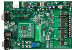
This low-voltage development board provides a cost-effective method of evaluating and developing sensed or sensorless Brushless DC (BLDC) motor and Permanent Magnet Synchronous
