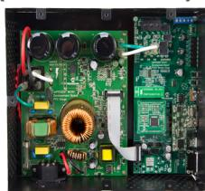
This high-voltage system is intended to aid the user in the rapid evaluation and development of a wide variety of motor control applications using a dsPIC DSC. This development system is targeted to control BLDC motors, PMSM and AC Induction
