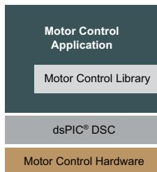
The Motor Control Library contains function blocks that are optimized for the dsPIC33F and dsPIC33E DSC families. All functions in this Motor Control Library have input(s) and output(s), but do not access any of the DSC peripherals. The library functions are designed to be used within an
