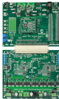
This bundle provides a cost-effective method of evaluating and developing dual/single motor control to drive BLDC motors or PMSMs concurrently, or one of each type of motor. The dsPIC DSC Signal Board supports both 3.3V and 5V devices for various applications and frequently used human interface includes some features and communication interfaces. The Motor Control 10–24V Driver Board (Dual/Single) supports currents up to 10A.
