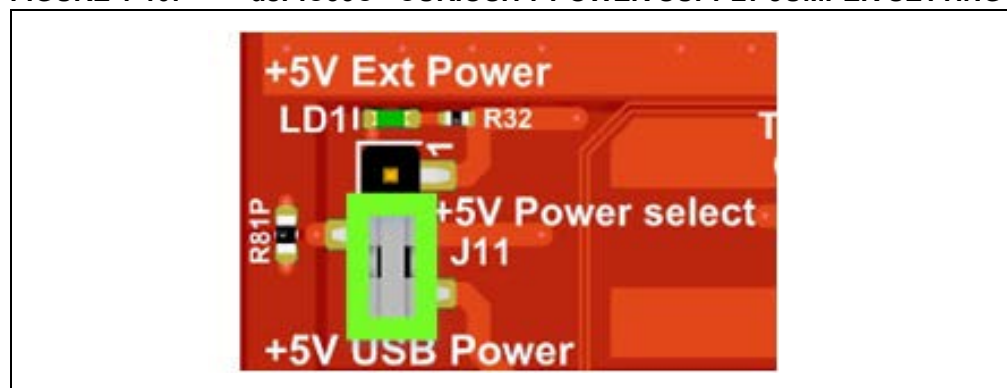
FIGURE 1-10: dsPIC33C® CURIOSITY POWER SUPPLY JUMPER SETTING
