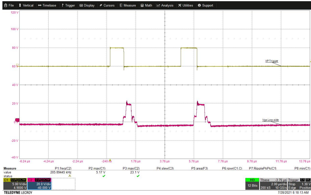
Figure 2-5. Minimum Double Pulse Waveform
