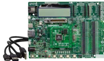
Explorer 16/32 Development Board with PIC24F1024GB610 Plug-In Module (DM240001-3)
