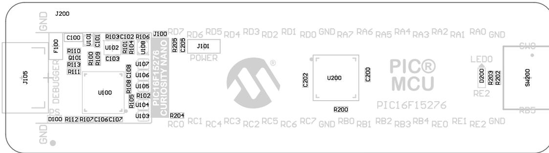
Figure 7-3. PIC16F15276 Curiosity Nano Assembly Drawing Bottom
