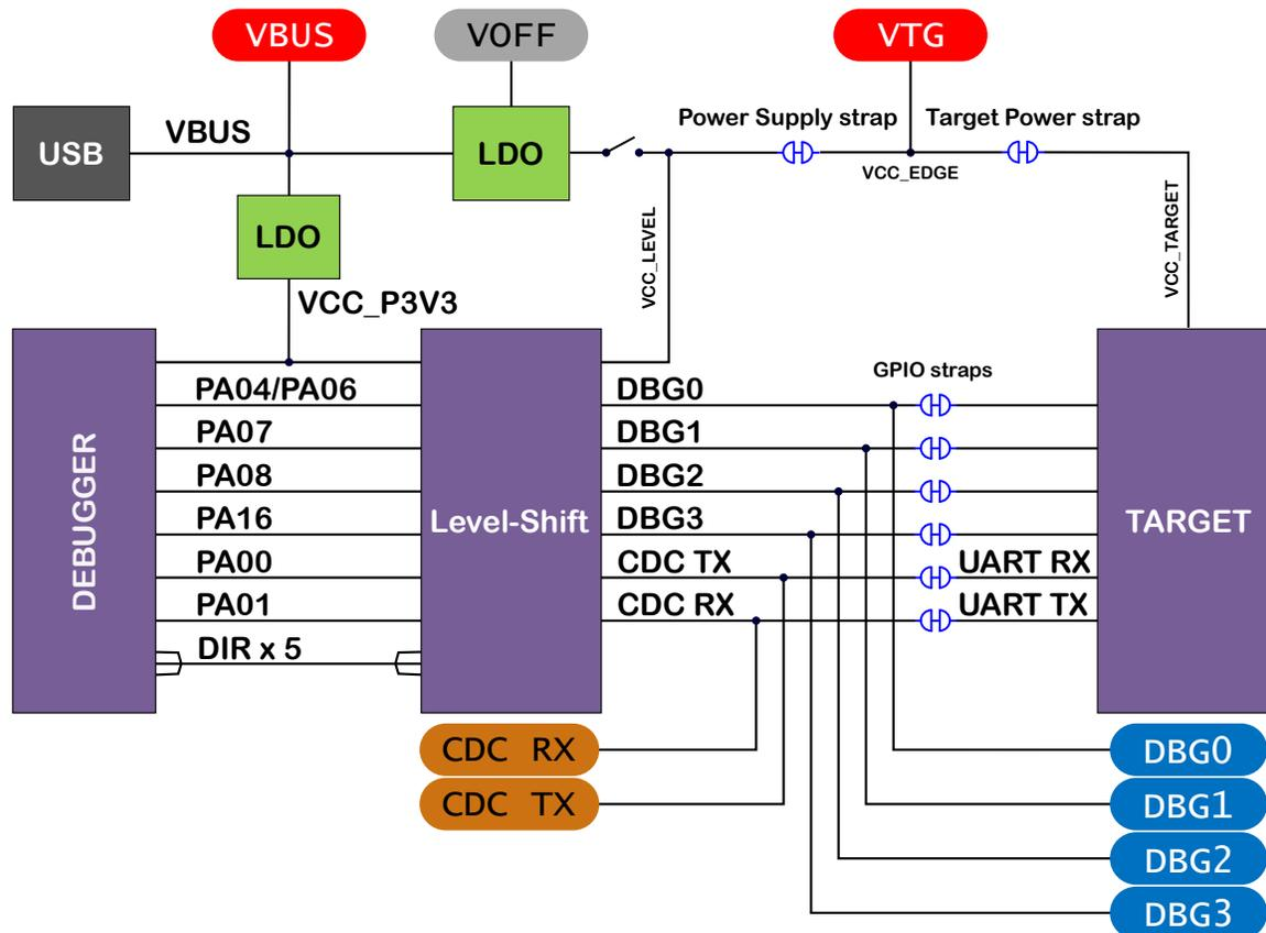
Figure 7-6. On-Board Debugger Connection Cut Straps
