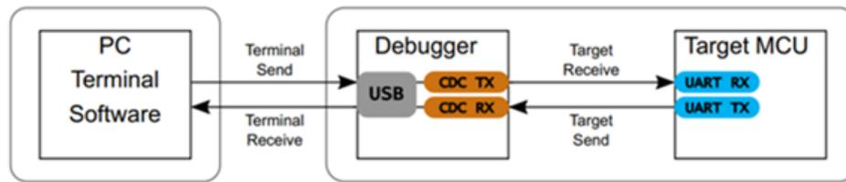
**Info:** As shown above, the CDC TX pin of the debugger is connected to a UART RX pin on the target for receiving characters from the Host computer. Similarly, the CDC RX pin of the debugger is connected to a UART TX pin on the target for transmitting characters to the Host computer.
