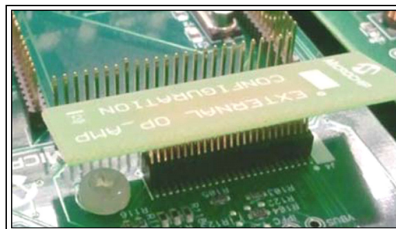
FIGURE 2: EXTERNAL OP AMP CONFIGURATION BOARD
