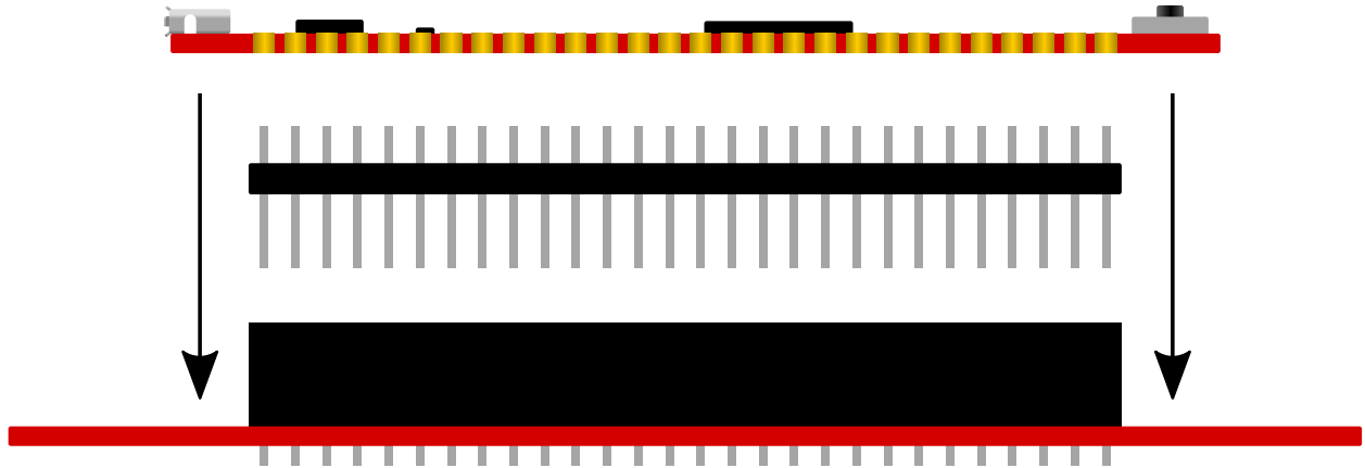
Figure 2-2. Connecting to Curiosity Nano Base for Click boards™
