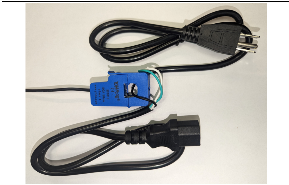
FIGURE 2-2: Current Transformer Connection.
