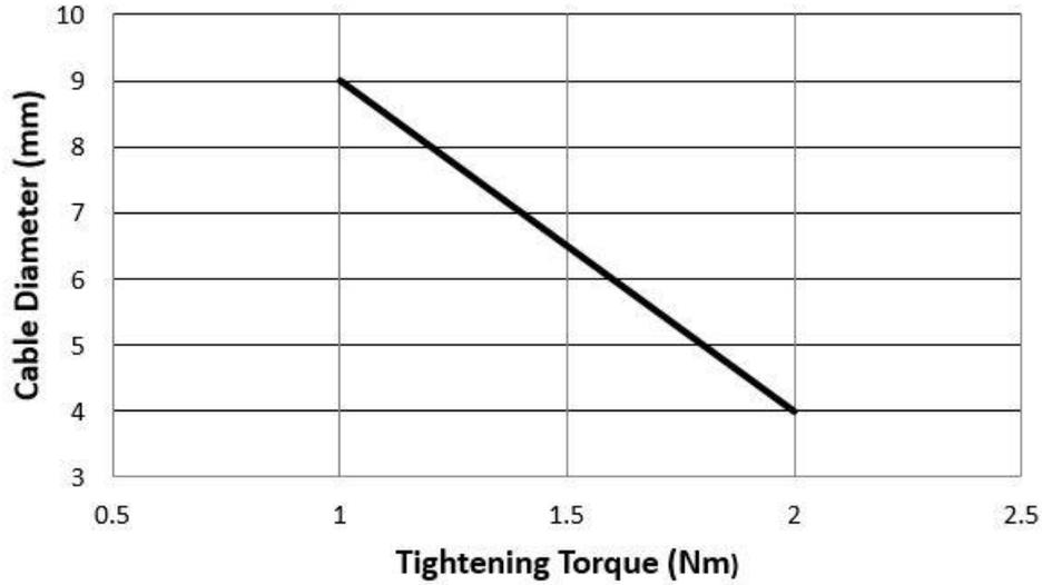
**Graph showing external thread tightening torque for Form A & B.**
