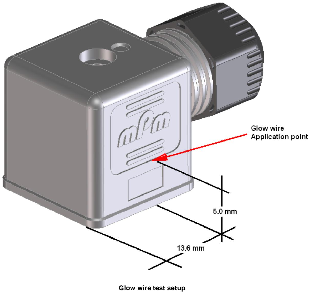
\*Note: height correct for form A, B and C.
