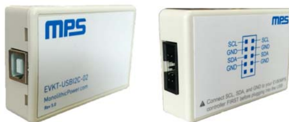
Figure 3: USB to I 2 C Communication Kit
