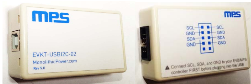
Figure 1: USB to I 2 C Communication Interface
