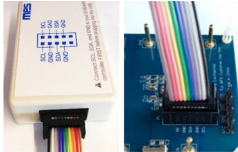
Figure 6: EVB to MPS I 2 C Communication Interface Wire Connection
