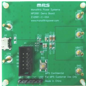
Figure 2: EV2661-C-00A Evaluation Board
