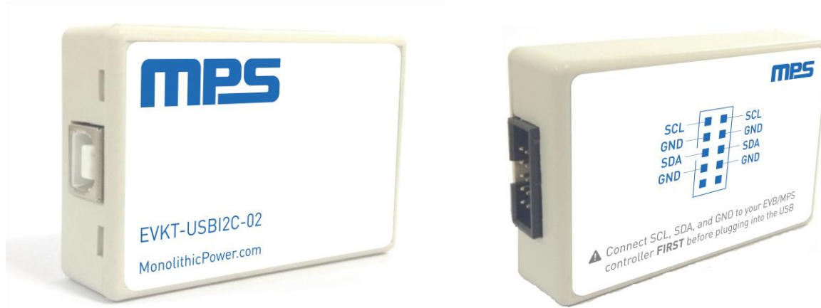
Figure 5: EVKT-USBI2C-02 Communication Interface
