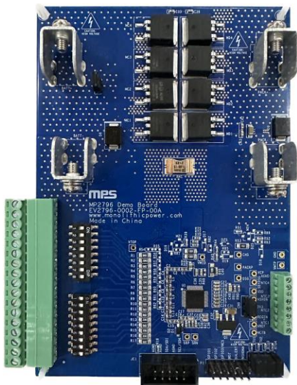
Figure 4: EV2796-0002-FP-00A Evaluation Board
