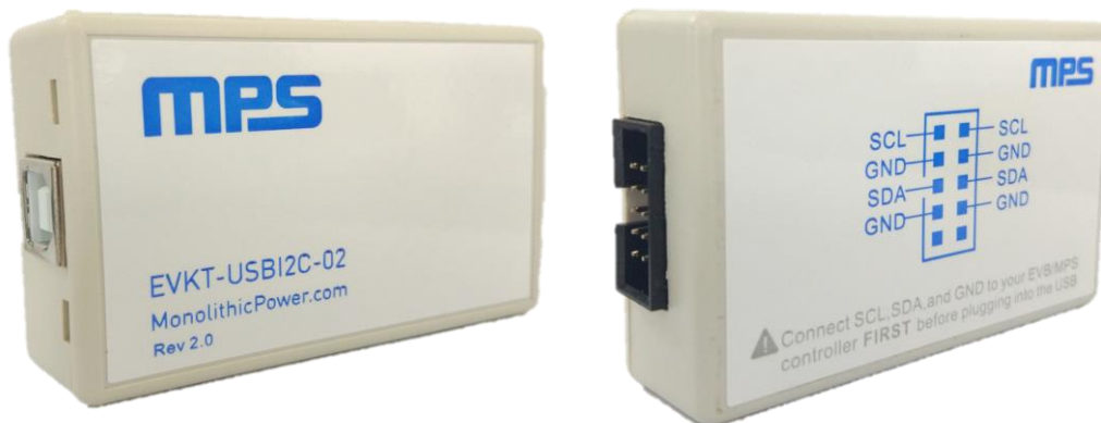
Figure 3: EVKT-USBI2C-02 Communication Interface
