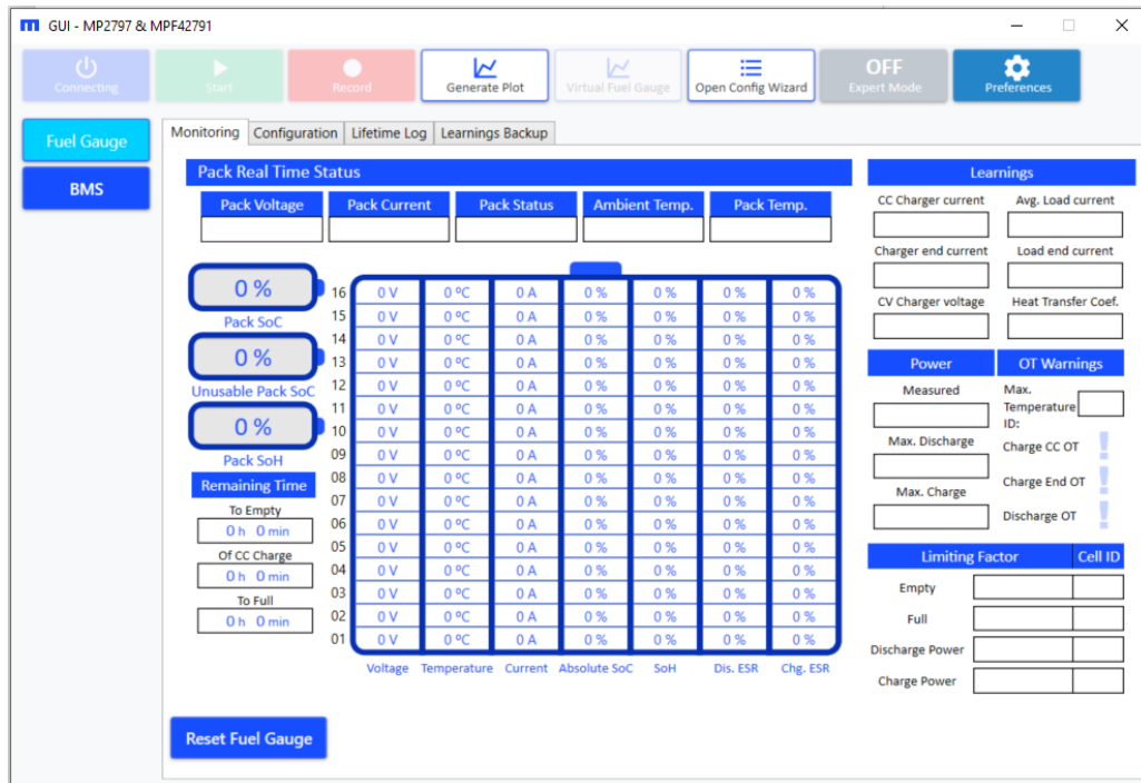
Figure 33: GUI Connecting to the BMUxxS-P100-x
