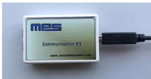
Figure 19: USB to UART Communication Interface (FT485R-KIT)
