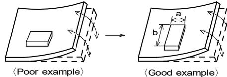
(2) Components location on PCB separation
