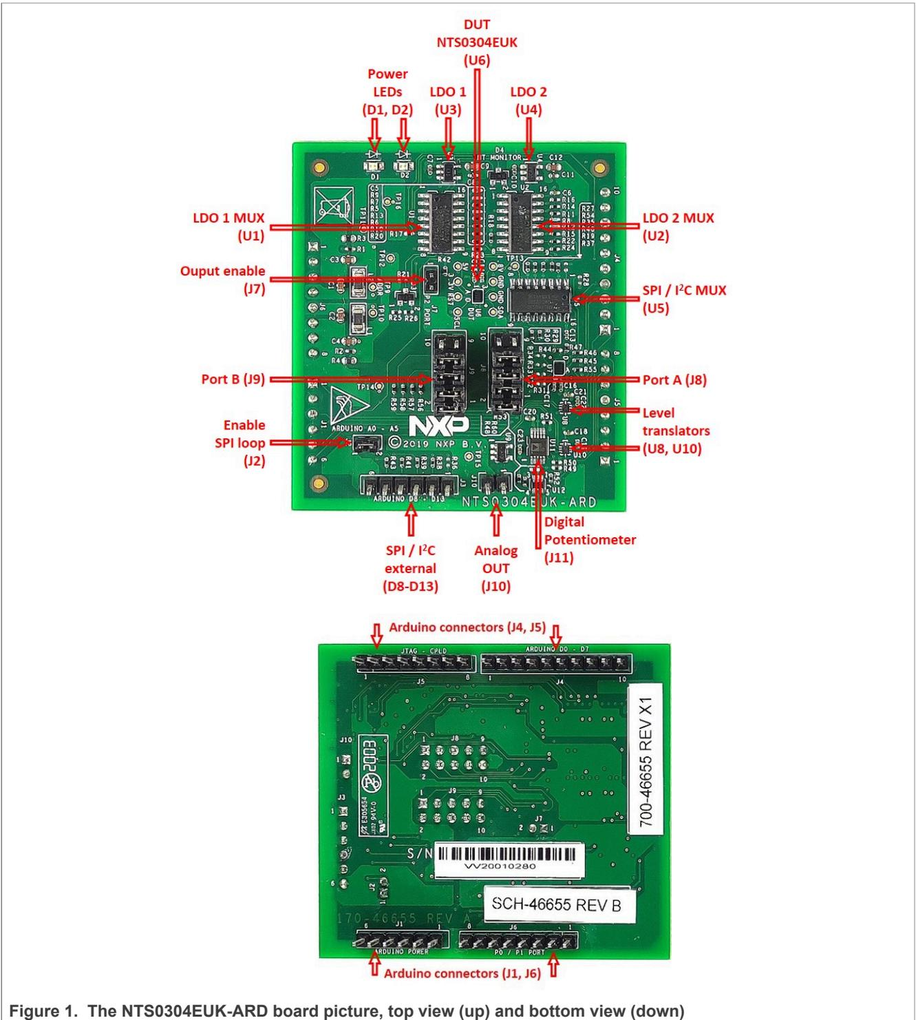
Figure 1. The NTS0304EUK-ARD board picture, top view (up) and bottom view (down)
