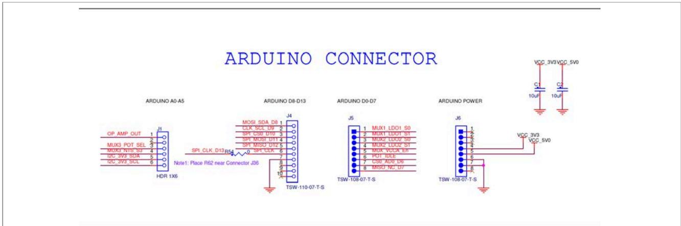
Figure 3. NTS0304EUK-ARD – Arduino connectors
