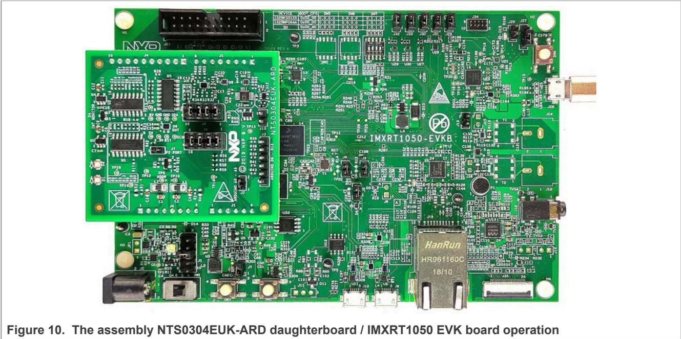
Figure 10. The assembly NTS0304EUK-ARD daughterboard / IMXRT1050 EVK board operation
