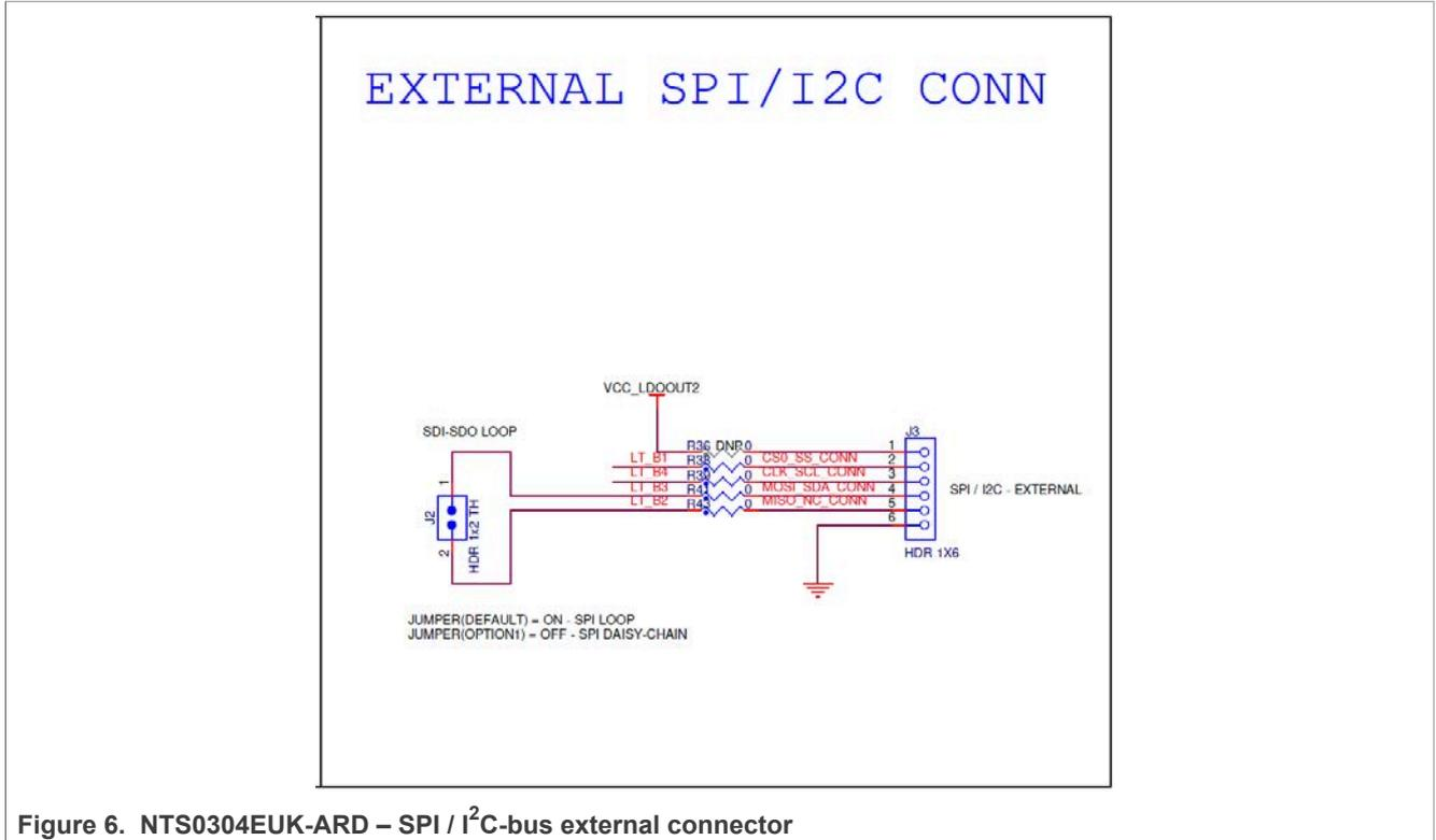
Figure 6. NTS0304EUK-ARD – SPI / I<sup>2</sup>C-bus external connector
