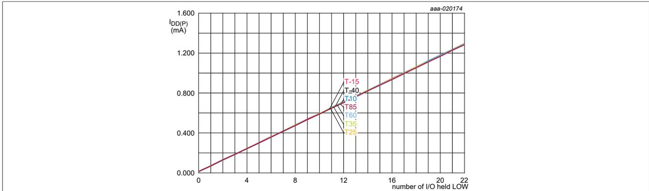
**Figure 23. Supply current versus number of I/O held LOW**
