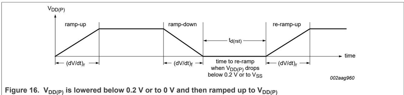
Figure 16. V<sub>DD(P)</sub> is lowered below 0.2 V or to 0 V and then ramped up to V<sub>DD(P)</sub>
