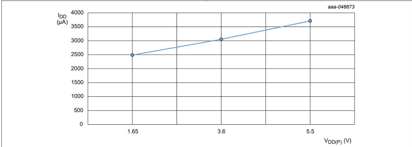
$T_{amb} = 25 \text{ }^\circ\text{C}$ ;  $I_{DD} = I_{DD(SPI)} + I_{DD(P)}$ ,  $f_{SCLK} = 5 \text{ MHz}$
