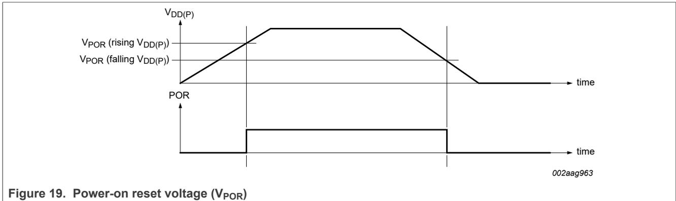
Figure 19. Power-on reset voltage ( $V_{POR}$ )
