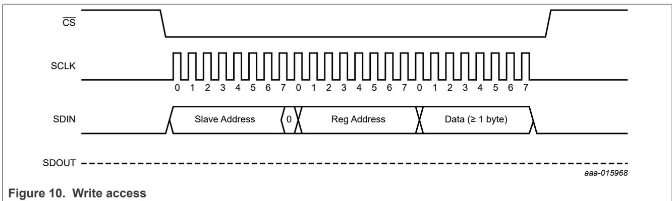
If more than 24 bits of data are transferred i.e. there are more than 24 clock pulses before de-asserting the CS, the register address is auto incremented. Auto Increment is discussed in a section below.
