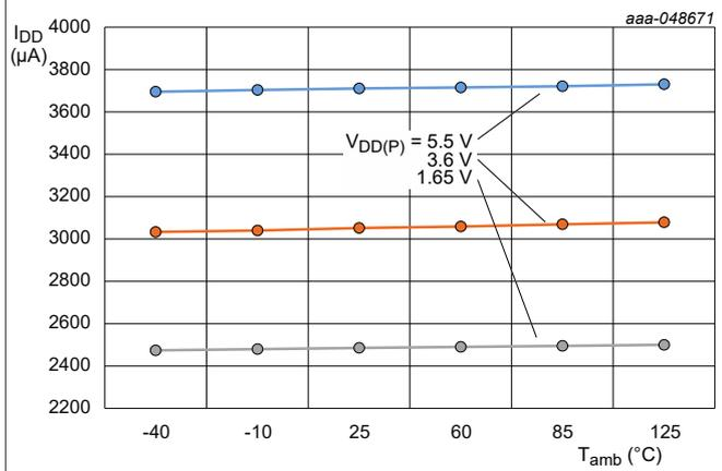
$I_{DD} = I_{DD(SPI)} + I_{DD(P)}$ ,  $f_{SCLK} = 5 \text{ MHz}$
