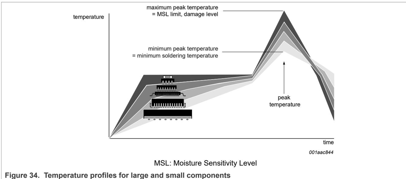
Figure 34. Temperature profiles for large and small components
