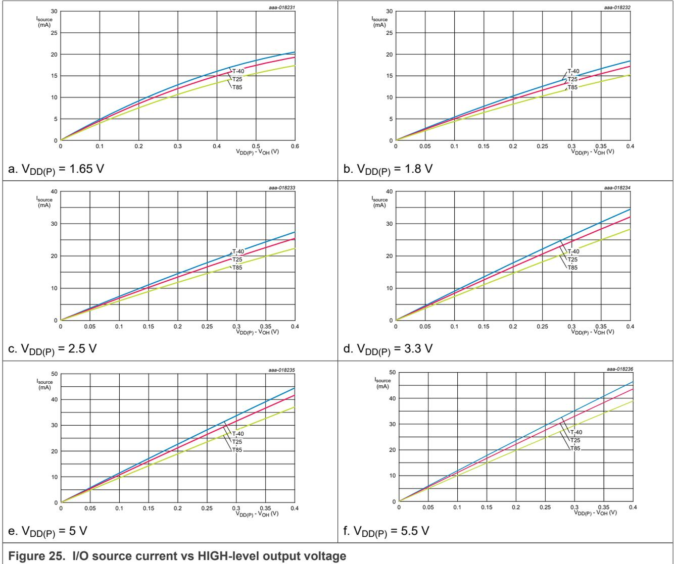
Figure 25. I/O source current vs HIGH-level output voltage
