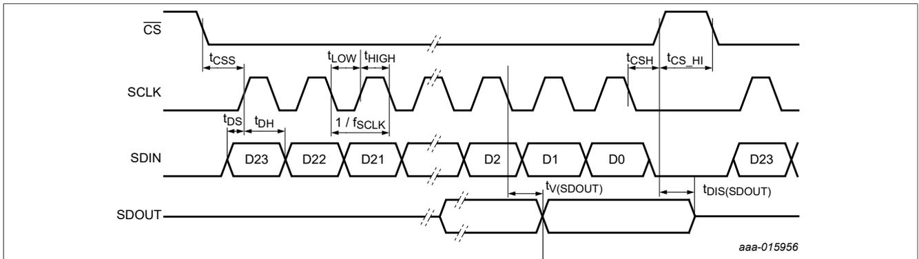
Figure 28. Definition of timing
