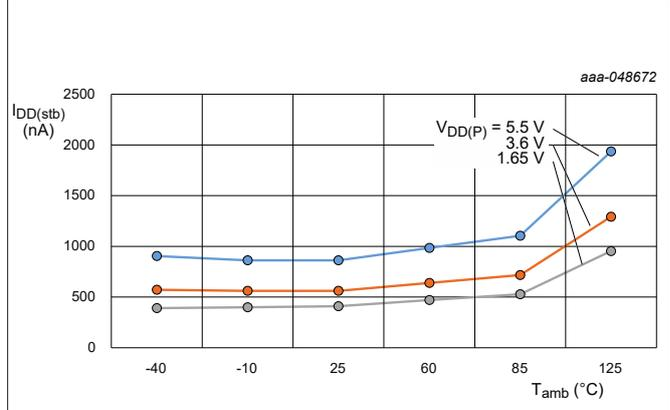
$I_{DD} = I_{DD(SPI)} + I_{DD(P)}$ ,  $f_{SCLK} = 0 \text{ Hz}$
