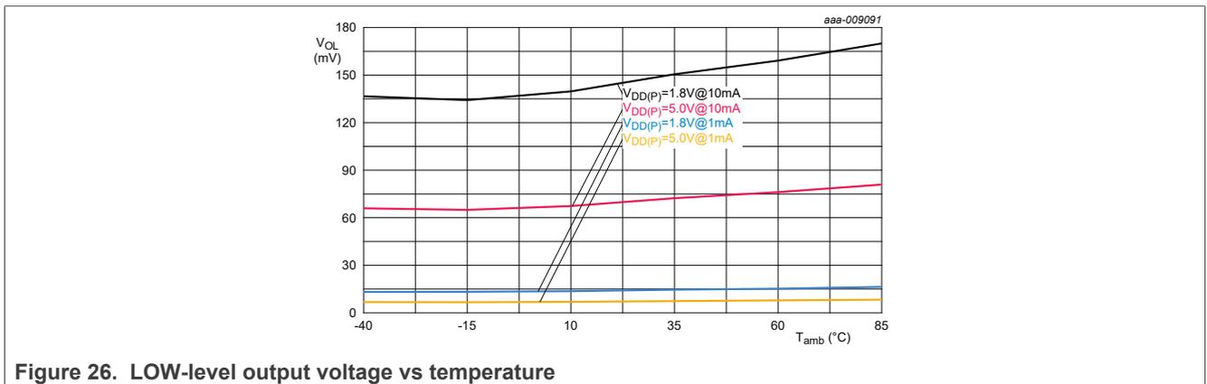
Figure 26. LOW-level output voltage vs temperature
