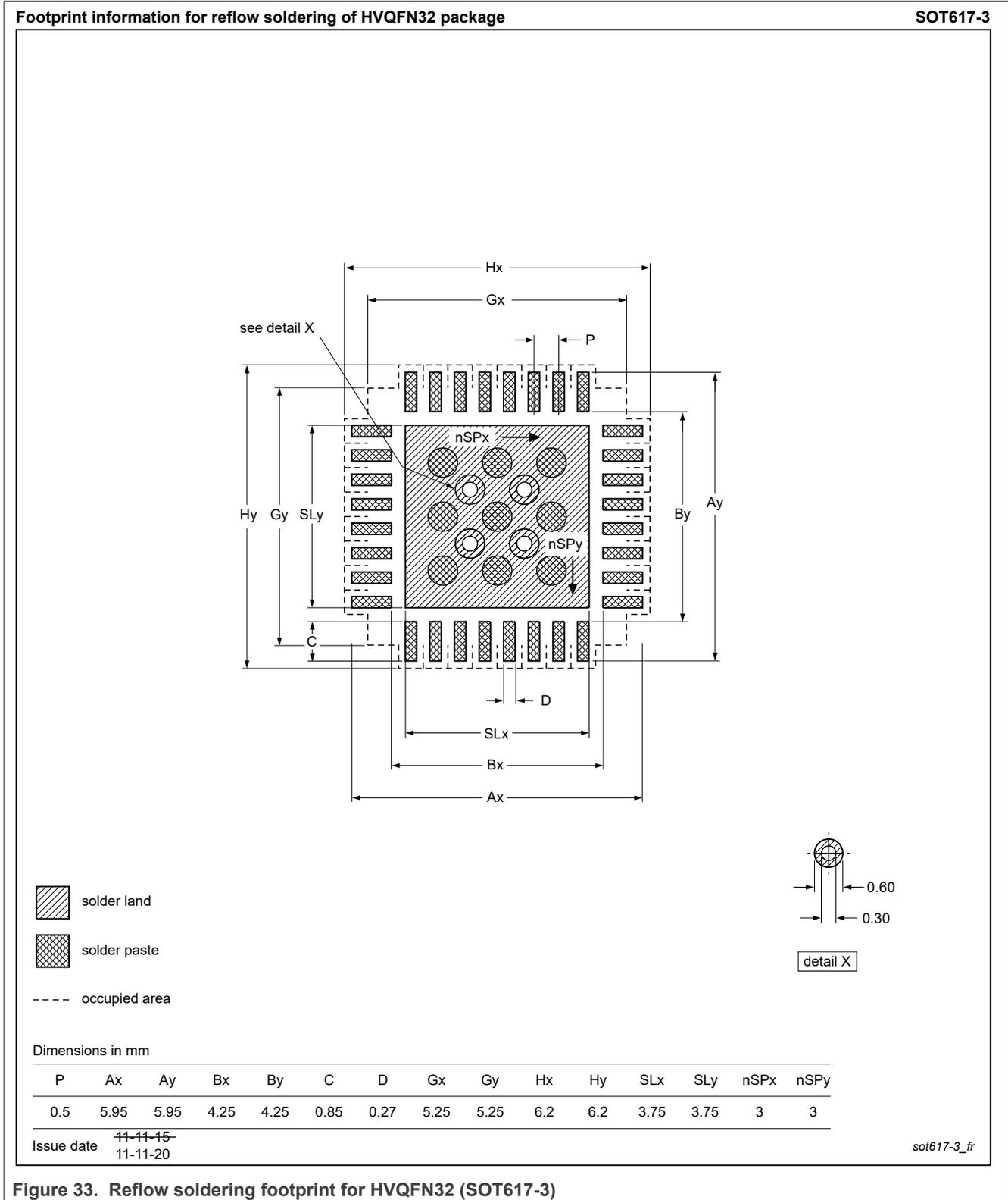
Figure 33. Reflow soldering footprint for HVQFN32 (SOT617-3)
