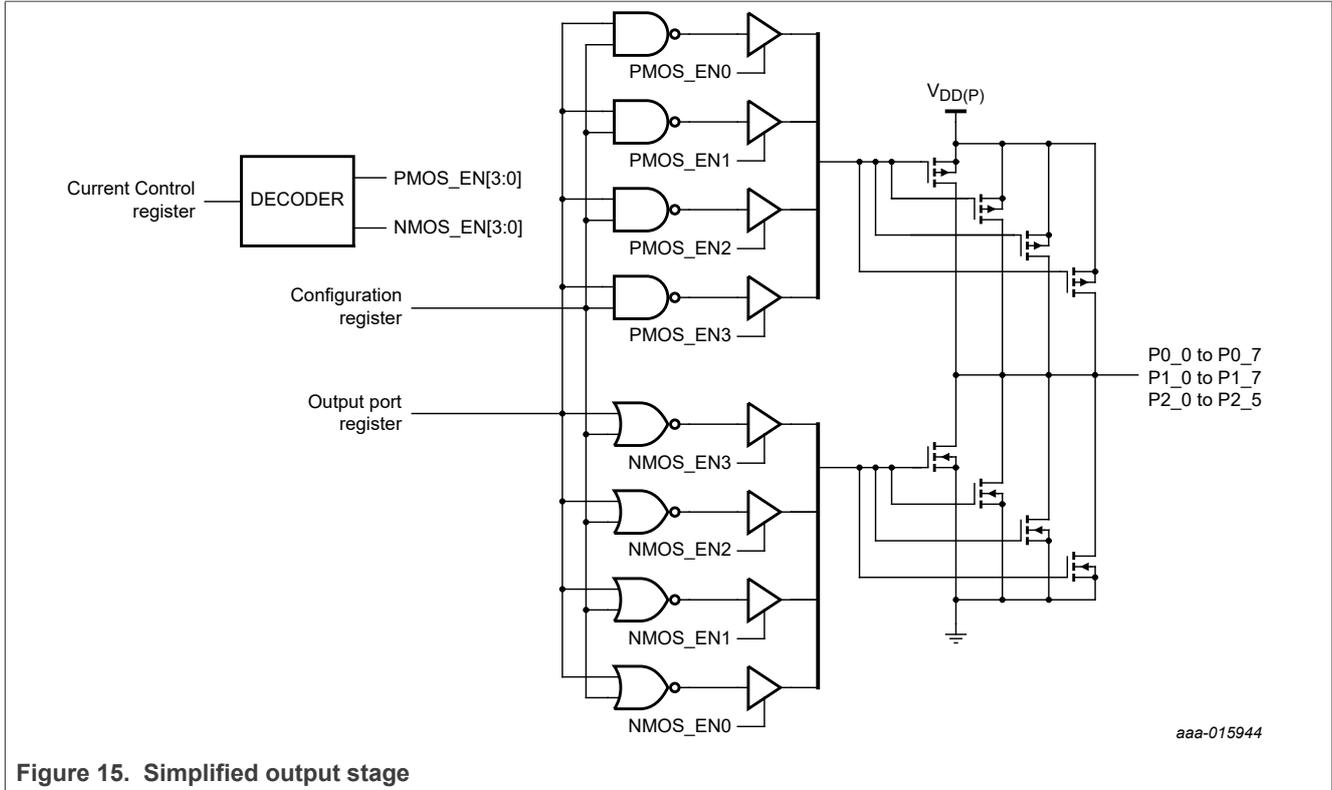
Figure 15. Simplified output stage
