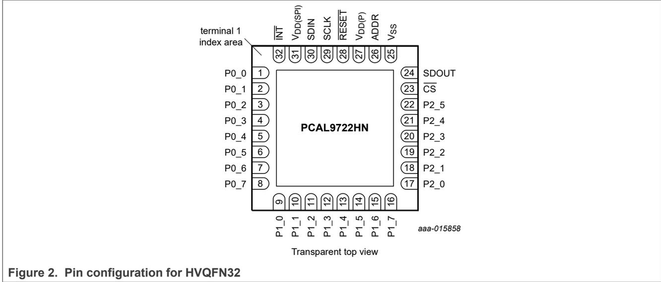
Figure 2. Pin configuration for HVQFN32
