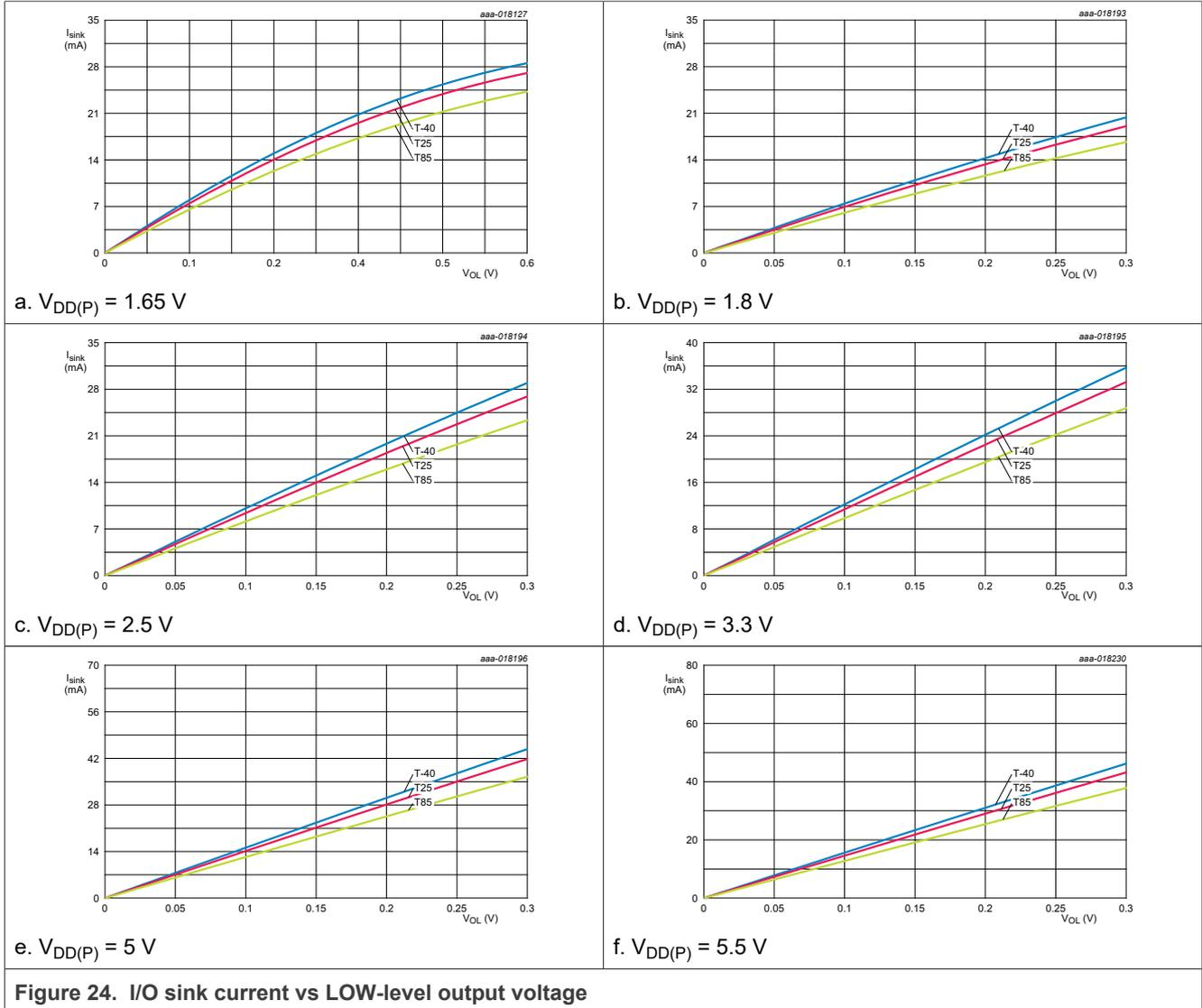
Figure 24. I/O sink current vs LOW-level output voltage
