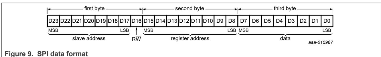
Figure 9. SPI data format
