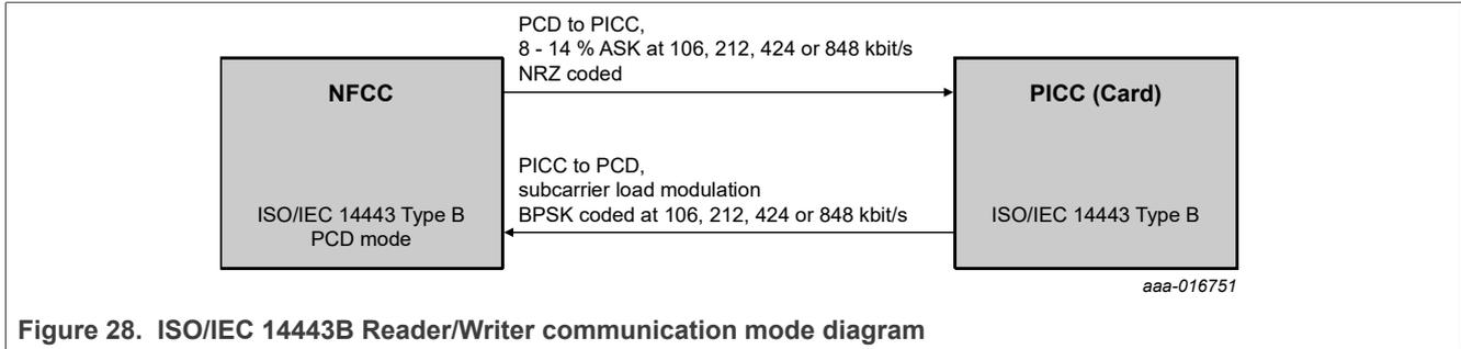
Figure 28. ISO/IEC 14443B Reader/Writer communication mode diagram
