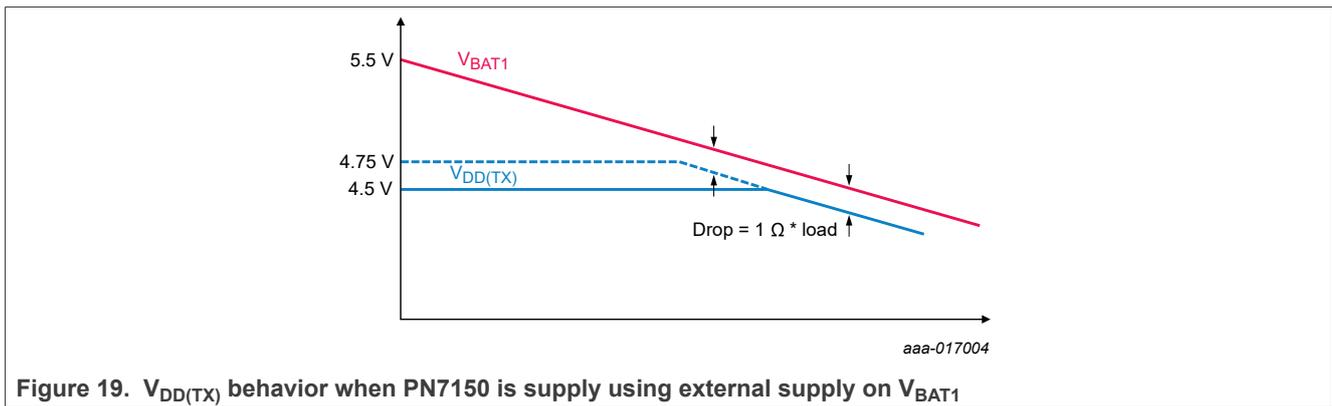
Figure 19 shows the behavior of  $V_{DD(TX)}$  depending on  $V_{BAT1}$  value.
