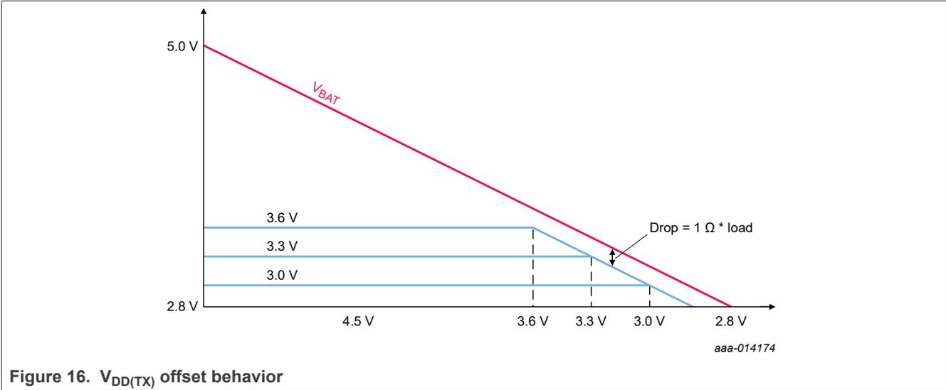
Figure 16 shows  $V_{DD(TX)}$  offset disabled behavior for both cases of  $V_{DD(TX)}$  programmed for 3.0 V, 3.3 V or 3.6 V.
