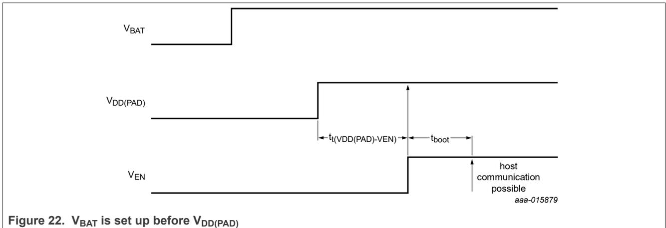
Figure 22.  $V_{BAT}$  is set up before  $V_{DD(PAD)}$
