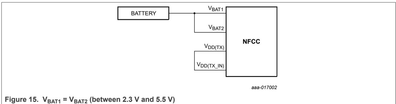
Figure 15.  $V_{BAT1} = V_{BAT2}$  (between 2.3 V and 5.5 V)
