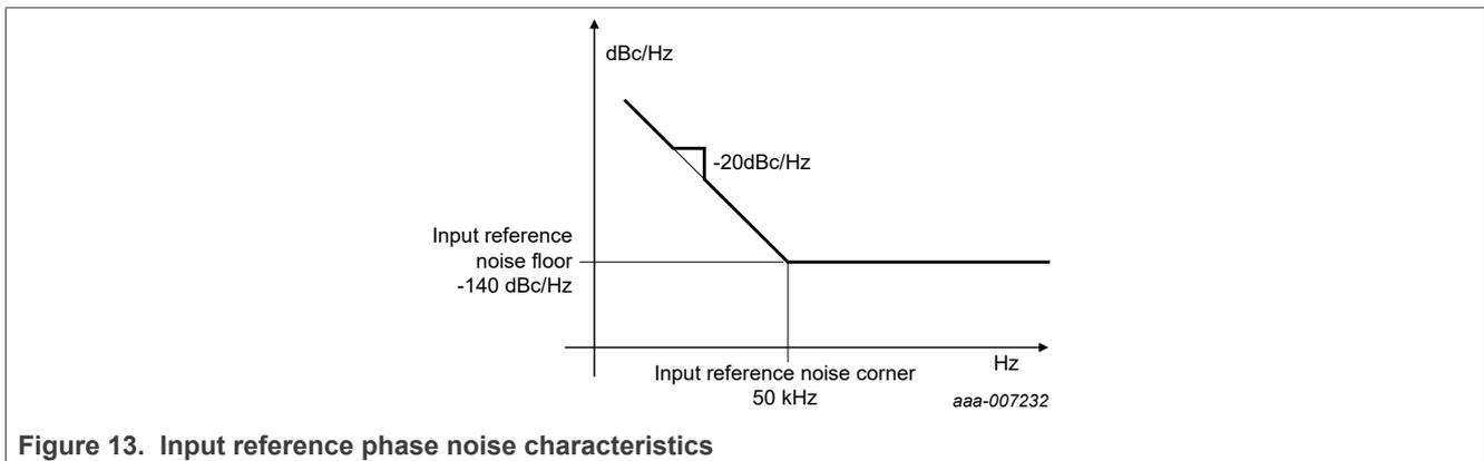
Figure 13. Input reference phase noise characteristics
