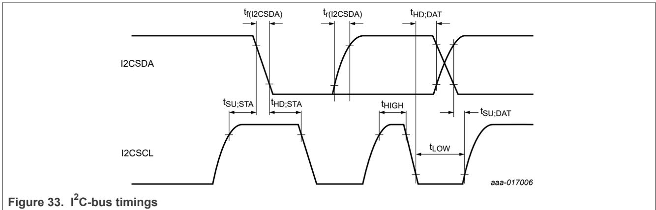
Figure 33. I<sup>2</sup>C-bus timings
