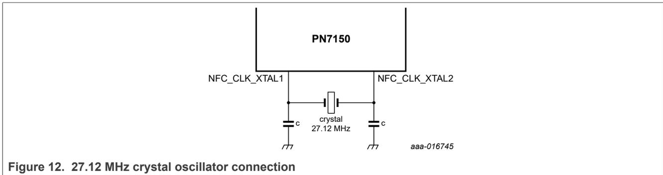
Figure 12. 27.12 MHz crystal oscillator connection
