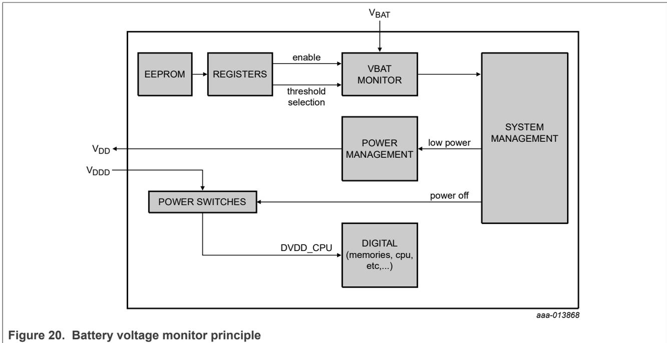
Figure 20. Battery voltage monitor principle
