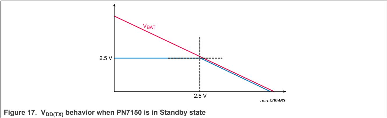
Figure 17 shows the case where the PN7150 is in standby state.
