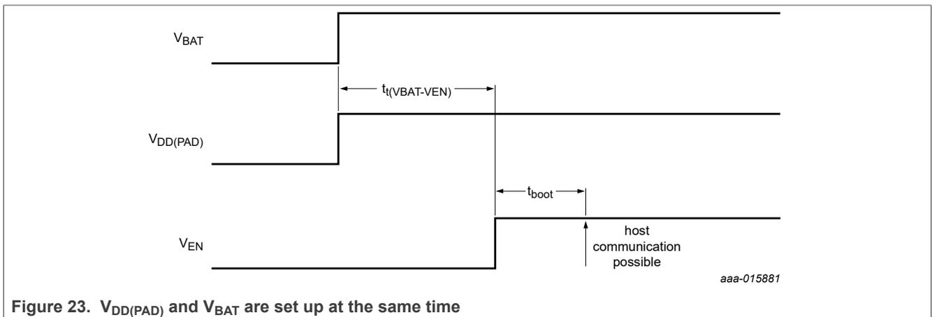
Figure 23.  $V_{DD(PAD)}$  and  $V_{BAT}$  are set up at the same time
