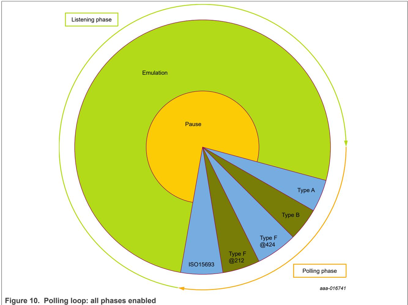
Listening phase uses Standby power state (when no RF field) and PN7150 goes to Listener mode when RF field is detected. When in Polling phase, PN7150 goes to Poller mode.
