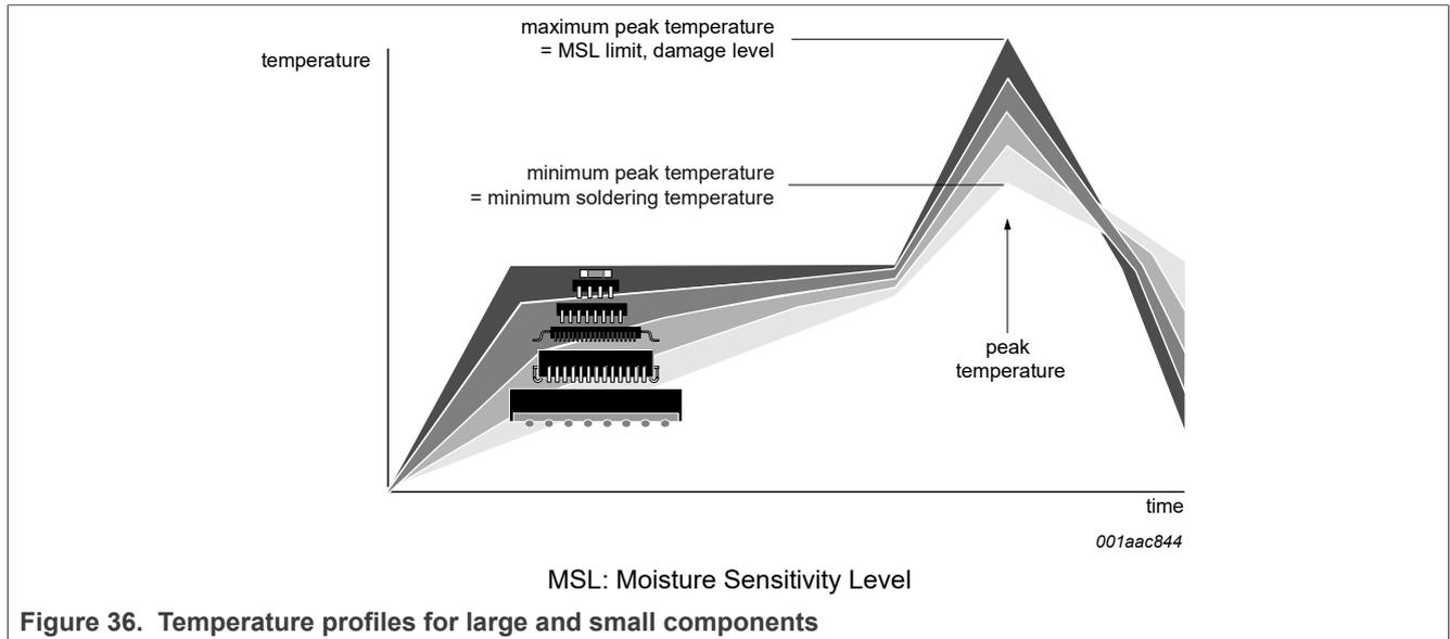
Figure 36. Temperature profiles for large and small components
