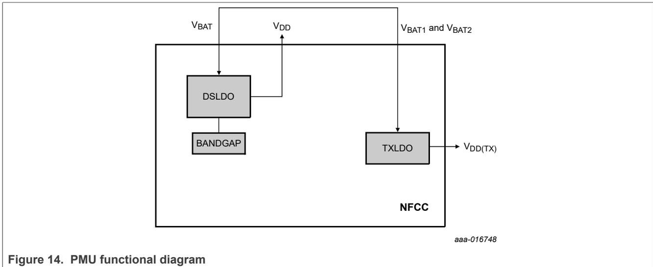
Figure 14. PMU functional diagram
