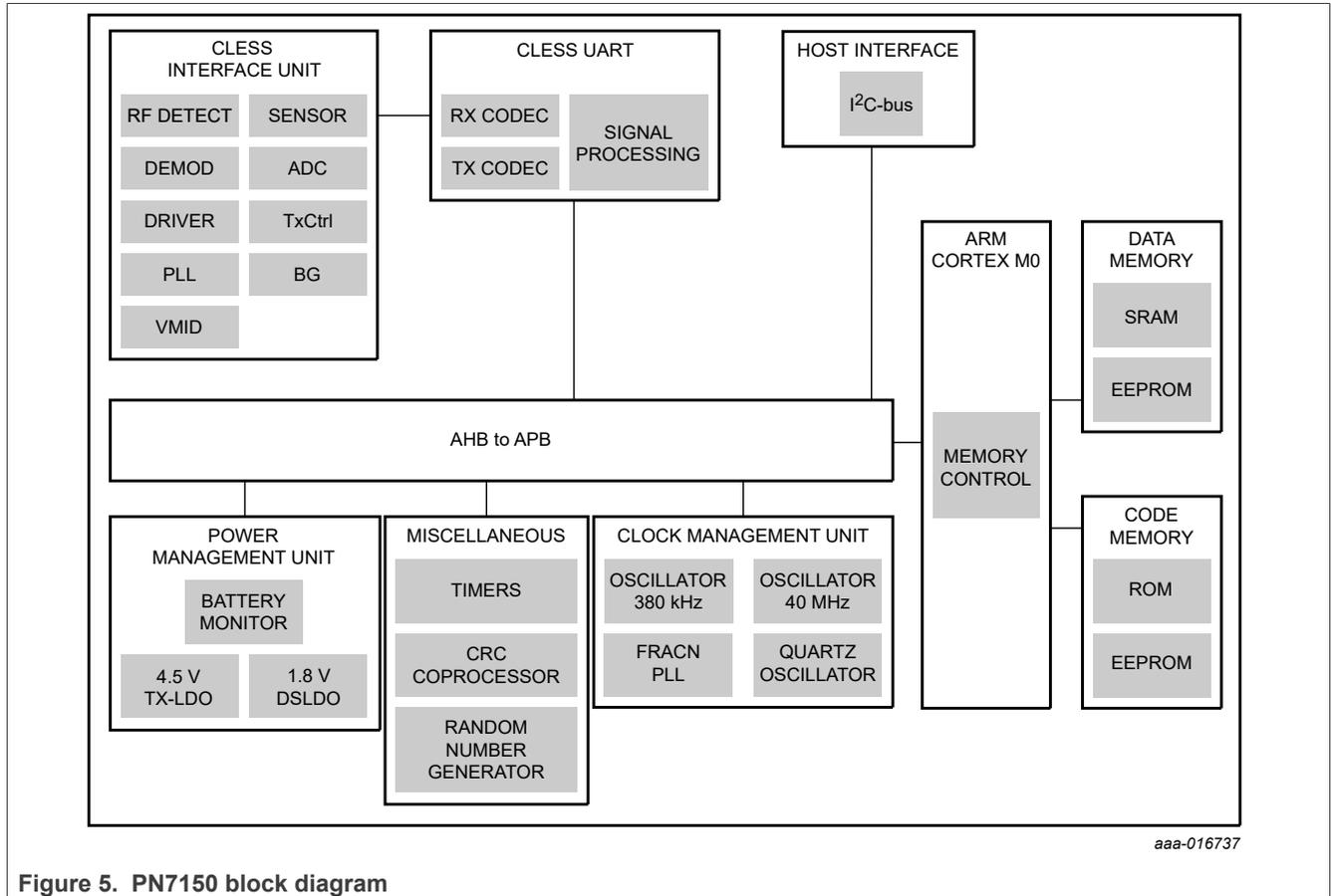
Figure 5. PN7150 block diagram
