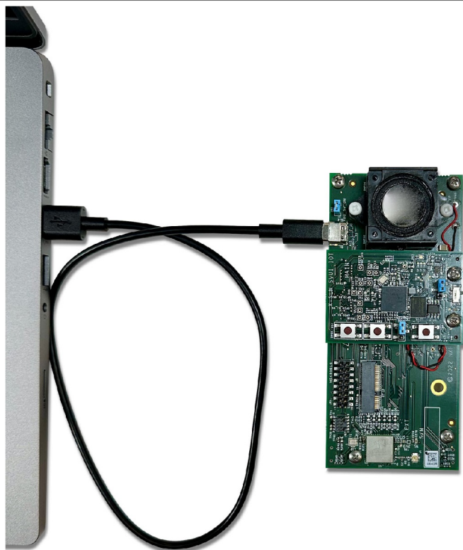
Figure 4. Connecting the SLN-SVUI-IOT Kit to the computer using a USB cable
