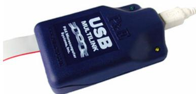
Figure 8-1: P&E's USB Multilink (USB-ML-PPCNEXUS shown)
