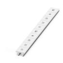
Marker for terminal blocks, Strip, white, labeled, can be labeled with: CMS-P1-PLOTTER, horizontal: L1, L2, L3, N, PE, L1, L2, L3, N, PE, mounting type: snapped, for terminal block width: 10.2 mm, lettering field size: 10,15 x 10,5 mm, Number of individual labels: 10
