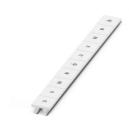
Marker for terminal blocks, Strip, white, labeled, can be labeled with: CMS-P1-PLOTTER, horizontal: U, V, W, N, GND, U, V, W, N, GND, mounting type: snapped, for terminal block width: 10.2 mm, lettering field size: 10,15 x 10,5 mm, Number of individual labels: 10
