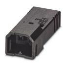
PCB connector, nominal cross section: 0.75 mm², color: black, nominal current: 6 A, rated voltage (III/2): 160 V, contact connection type: Pin, number of potentials: 2, number of rows: 1, number of positions: 2, number of connections: 2, product range: PTCM 0,5/..-PI, pitch: 2.5 mm, connection method: Crimp connection, conductor/PCB connection direction: 0 °, plug-in system: COMBICON PTSM, locking: Snap-in locking, mounting: Engagement nose, type of packaging: packed in cardboard
