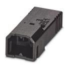
PCB connector, nominal cross section: 0.75 mm², color: black, nominal current: 6 A, rated voltage (III/2): 160 V, contact connection type: Pin, number of potentials: 6, number of rows: 1, number of positions: 6, number of connections: 6, product range: PTCM 0,5/..-PI, pitch: 2.5 mm, connection method: Crimp connection, conductor/PCB connection direction: 0 °, plug-in system: COMBICON PTSM, locking: Snap-in locking, mounting: Engagement nose, type of packaging: packed in cardboard
