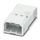
PCB connector, nominal cross section: 0.75 mm², color: white, nominal current: 6 A, rated voltage (III/2): 160 V, contact connection type: Pin, number of potentials: 4, number of rows: 1, number of positions: 4, number of connections: 4, product range: PTCM 0,5/..-PI, pitch: 2.5 mm, connection method: Crimp connection, conductor/PCB connection direction: 0 °, plug-in system: COMBICON PTSM, locking: Snap-in locking, mounting: Engagement nose, type of packaging: packed in cardboard
