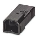
PCB connector, nominal cross section: 0.75 mm², color: black, nominal current: 6 A, rated voltage (III/2): 160 V, contact connection type: Pin, number of potentials: 6, number of rows: 1, number of positions: 6, number of connections: 6, product range: PTCM 0,5/..-PI, pitch: 2.5 mm, connection method: Crimp connection, conductor/PCB connection direction: 0 °, plug-in system: COMBICON PTSM, locking: Snap-in locking, mounting: Engagement nose, type of packaging: packed in cardboard
