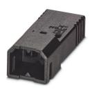
PCB connector, nominal cross section: 0.75 mm², color: black, nominal current: 6 A, rated voltage (III/2): 160 V, contact connection type: Pin, number of potentials: 8, number of rows: 1, number of positions: 8, number of connections: 8, product range: PTCM 0,5/..-PI, pitch: 2.5 mm, connection method: Crimp connection, conductor/PCB connection direction: 0 °, plug-in system: COMBICON PTSM, locking: Snap-in locking, mounting: Engagement nose, type of packaging: packed in cardboard
