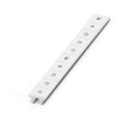
Marker for terminal blocks, Strip, white, labeled, can be labeled with: CMS-P1-PLOTTER, horizontal: L1, L2, L3, N, PE, L1, L2, L3, N, PE, mounting type: snapped, for terminal block width: 10.2 mm, lettering field size:  $10,15 \times 10,5$  mm, Number of individual labels: 10
