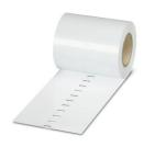
Marker for terminal blocks, Roll, white, unlabeled, can be labeled with: THERMOMARK ROLL 2.0, THERMOMARK ROLL, THERMOMARK ROLL X1, THERMOMARK ROLLMASTER 300/600, THERMOMARK X1.2, THERMOMARK S1.1, perforated, mounting type: snapped, snap into flat marker groove, for terminal block width: 10.2 mm, lettering field size: 6.35 x 10.15 mm, Number of individual labels: 10000
