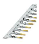
Crimp contact, Pin, rolled, Taped product, number of pieces per reel: 500, contact diameter: 1 mm, crimp range: 0.22 mm $^2$  ... 0.56 mm $^2$ , Item is lead-free in accordance with RoHS II without Exemption 6c (Pb < 0.1 %)
