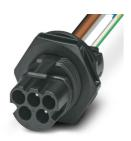
Device connector rear mounting, Range of articles: PRC 35, housing material: PPE, color: black, number of positions: 5, max. conductor cross section: 4 mm², rated voltage: 690 V AC, rated current: 32 A, Connection method: Crimp connection, Contact connection type: Pin, cable length: 150, This item is also available with other cable lengths. For your specific requirements, please contact your local PHOENIX CONTACT subsidiary.
