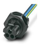
Device connector rear mounting, Range of articles: PRC 35, housing material: PPE, color: black, number of positions: 3, max. conductor cross section: 4 mm², rated voltage: 690 V AC, rated current: 32 A, Connection method: Crimp connection, Contact connection type: Pin, cable length: 150, This item is also available with other cable lengths. For your specific requirements, please contact your local PHOENIX CONTACT subsidiary.
