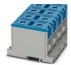
High-current terminal block, nom. voltage: 1000 V, nominal current: 290 A, number of connections: 2, number of positions: 1, connection method: Screw connection, Rated cross section: 150 mm<sup>2</sup>, cross section: 35 mm<sup>2</sup> - 150 mm<sup>2</sup>, Rated cross section: 150 mm<sup>2</sup>, cross section: 35 mm<sup>2</sup> - 150 mm<sup>2</sup>, mounting type: NS 35/15, NS 35/7,5, color: blue
