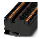
Fuse modular terminal block, fuse type: Flat, fuse type: C, nom. voltage: 24 V, nominal current: 25 A, connection method: Push-in connection, Rated cross section: 10 mm<sup>2</sup>, cross section: 0.5 mm<sup>2</sup>- 16 mm<sup>2</sup>, mounting type: NS 35/7,5, NS 35/15, color: black
