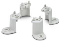
Adapter for mounting the UCS housing on the wall, material: polyamide, color: light gray similar to RAL 7035, used instead of UCS CC corner insert; only used in conjunction with UCS GD 9005 adhesive pad
