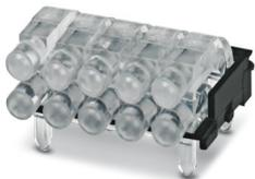
Multiple light guides with glare protection, passive, rigid, Raised head, Emission surface: spherical, Number of displays: 10, (2 rows, 5 columns), pitch: 2.54 mm, ESD protection: <8 kV, can be used for the ME, ME-MAX, ME-IO, ME PLC, and EH housing ranges (housing must be processed)
