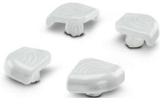
Adapter for protecting the corners of the UCS housing; material: TPE-U; color: light gray, similar to RAL 7035; held in the screw holes of the housing
