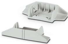
Stand for mounting the UCS housing; height: 47 mm; material: polyamide; color: light gray, similar to RAL 7035; wall mounting option is integrated, snaps into the screw holes of the housing
