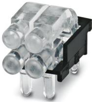
Multiple light guides with glare protection, passive, rigid, Raised head, Emission surface: spherical, Number of displays: 4, (2 rows, 2 columns), pitch: 2.54 mm, ESD protection: <8 kV, can be used for the ME, ME-MAX, ME-IO, ME PLC, and EH housing ranges (housing must be processed)
