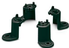
Adapter for mounting the UCS housing on the wall, material: polyamide, color: black similar to RAL 9005, used instead of UCS CC corner insert; only used in conjunction with UCS GD 9005 adhesive pad
