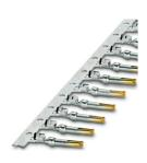
Crimp contact, Socket, rolled, Taped product, number of pieces per reel: 10000, contact diameter: 1 mm, crimp range: 0.22 mm $^2$  ... 0.56 mm $^2$ , Item is lead-free in accordance with RoHS II without Exemption 6c (Pb < 0.1 %)
