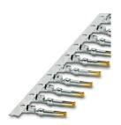
Crimp contact, Socket, rolled, Taped product, number of pieces per reel: 500, contact diameter: 1 mm, crimp range: 0.22 mm $^2$  ... 0.56 mm $^2$ , Item is lead-free in accordance with RoHS II without Exemption 6c (Pb < 0.1 %)
