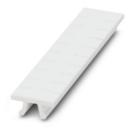
Zack marker strip, Strip, white, unlabeled, can be labeled with: PLOTMARK, CMS-P1-PLOTTER, mounting type: snapped, for terminal block width: 5.08 mm, lettering field size: 4.98 x 10.5 mm, Number of individual labels: 10
