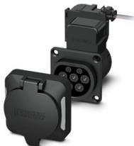
CHARX connect modular, Infrastructure charging socket, square, Premium, Set, with square protective cover, with temperature sensors, with LED (common cathode connection), for charging electric vehicles (EV) with alternating current (AC), Type 2, IEC 62196-2, 32 A / 480 V (AC), without single-core wires, locking actuator: 12 V, 3-pos., Rear panel mounting, M5 thread, housing: black, PHOENIX CONTACT logo
