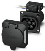
CHARX connect modular, Infrastructure charging socket, square, Premium, Set, with square protective cover, with temperature sensors, with LED (common cathode connection), for charging electric vehicles (EV) with alternating current (AC), Type 2, IEC 62196-2, 32 A / 480 V (AC), without single-core wires, locking actuator: 12 V, 4-pos., Rear panel mounting, M5 thread, housing: black, PHOENIX CONTACT logo
