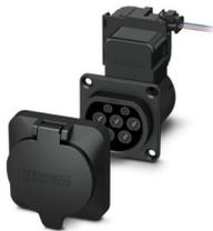
CHARX connect modular, Infrastructure charging socket, square, Basic, Set, with square protective cover, for charging electric vehicles (EV) with alternating current (AC), Type 2, IEC 62196-2, 32 A / 480 V (AC), without single-core wires, locking actuator: 12 V, 3-pos., Rear panel mounting, M5 thread, housing: black, PHOENIX CONTACT logo
