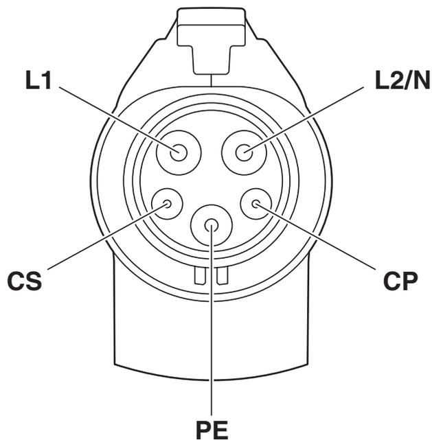
Pin assignment of the Vehicle Connector
