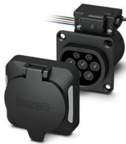
CHARX connect modular, Infrastructure charging socket, square, Basic, Set, with square protective cover, with LED (common cathode connection), for charging electric vehicles (EV) with alternating current (AC), Type 2, IEC 62196-2, 32 A / 480 V (AC), without single-core wires, locking actuator: 12 V, 4-pos., Rear panel mounting, M5 thread, housing: black, PHOENIX CONTACT logo
