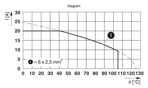
I = current strength,  $\vartheta$  = ambient temperature, 6x 20 A
