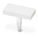
Marker for terminal blocks, Stud, white, unlabeled, can be labeled with: Marker pen, mounting type: plug in, for terminal block width: 7.5 mm, lettering field size:  $4 \times 7.5$  mm
