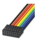
Power connector for DIN rail bus connector with 16 free cable ends with a cross section of 0.25 mm<sup>2</sup>, 500 mm long, female contacts
