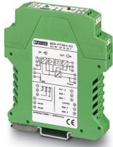
MCR temperature transducer, for Pt 100, 2-, 3-, 4-conductor technology; input: 0 ... 100°C, 0 ... 150°C, 0 ... 200°C, 0 ... 300°C, -50 ... +50°C, -50 ... 100°C, -50 ... 150°C, -50 ... 250°C, output signal: 0 ... 10 V, electrically isolated auxiliary power
